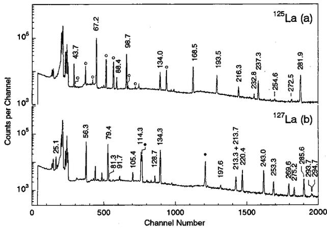
FIG. 1. Low energy portions of the  $\gamma$ -ray spectra in the decay of  $^{125}\text{La}$  (a) and  $^{127}\text{La}$  (b) obtained with a LEPS. The open and closed circles indicate the  $\gamma$  rays associated with the decay of their daughter or granddaughter nuclei, respectively.
