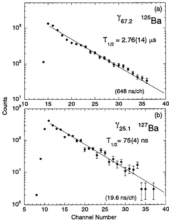
FIG. 2. Time distribution curves of the 67.2- and 25.1-keV  $\gamma$  transitions in the decays of  $^{125}\text{La}$  (a) and  $^{127}\text{La}$  (b), respectively.
