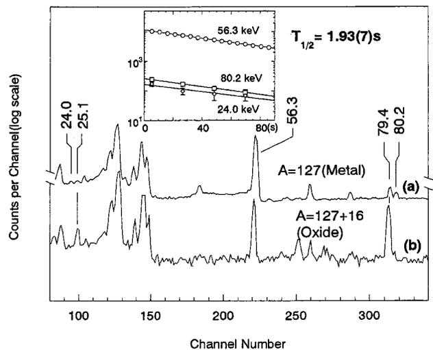
FIG. 4. Comparison of the  $\gamma$ -ray spectra obtained with a metallic beam [ $A=127$  (a)] and an oxide beam [ $A=127+16$  (b)]. The inset shows decay curves of the 80.2-, 56.3-, and 24.0-keV  $\gamma$  rays of the  $^{127m}\text{Ba}$  isomeric transitions.
