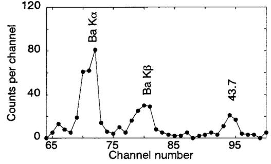
FIG. 6. Low energy portion of the coincident spectrum obtained with the LEPS gated by the 281.9-keV  $\gamma$  ray and  $\beta^+$  ray.
