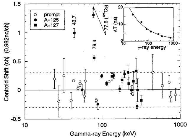
FIG. 3. Peak centroid shifts of  $\gamma$  transitions obtained with mass-separated beams of  $A=125+16$ ,  $127+16$  and prompt time distributions obtained by the external conversion technique. The inset shows the typical time resolution in this experiment.
