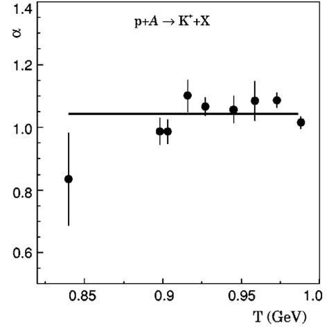
FIG. 1. Dependence of the parameter  $\alpha$  on the beam energy  $T_p$  evaluated from the PNPI data [1] on total  $K^+$ -production cross sections. The solid line indicates the fitted average value  $\alpha = 1.04 \pm 0.01$ .
