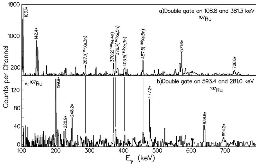
FIG. 2. (a) Upper panel: Coincidence spectrum obtained by double gates on the 108.8 and 381.3 keV transitions in  $^{107}\text{Ru}$ . (b) Lower panel: Coincidence spectrum obtained by a double gate on the 593.4 and 281.0 keV transitions in  $^{107}\text{Ru}$ .
