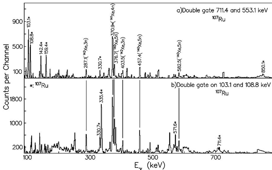
FIG. 3. (a) Upper panel: Coincidence spectrum obtained by double gates on the 711.4 and 553.1 keV transitions in  $^{107}\text{Ru}$ . (b) Lower panel: Coincidence spectrum obtained by a double gate on the 103.1 and 108.8 keV transitions in  $^{107}\text{Ru}$ .
