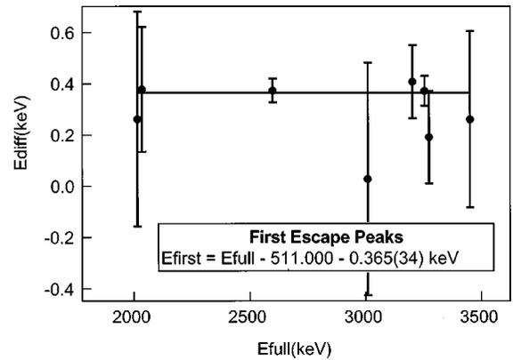
FIG. 8. The energies of eight first escape peaks from  $^{56}\text{Co}$ , in terms of the full energies minus 511.000 keV. The continuous line is the best fit to the points as a constant, independent of the full energy.
