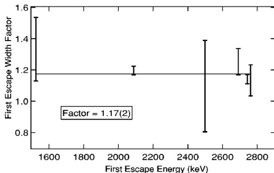
FIG. 7. The multiplying factor for the width parameter for six first escape peaks from  $^{56}\text{Co}$ . The continuous line is the best fit to the points as a constant, independent of the full energy.
