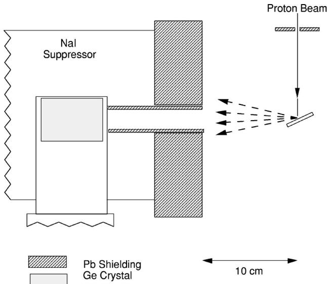
FIG. 2. A plan view of the experimental arrangement.
