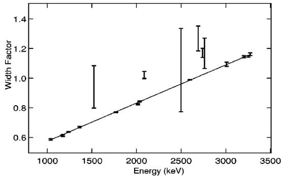
FIG. 6. The width parameter for all the lines of  $^{56}\text{Co}$  from 1.06 to 3.27 MeV, and the fit to this in terms of a parabolic function of the line energy. The six points above the line are from first escape peaks.
