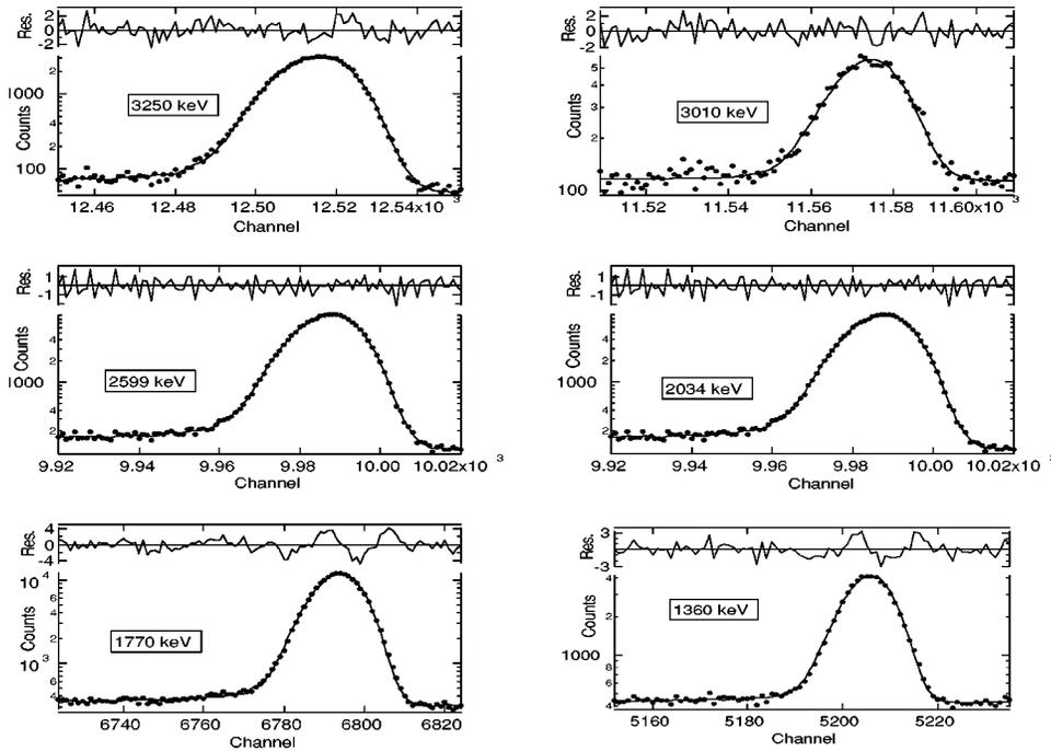
FIG. 3. Fits to the shapes of the  $^{56}\text{Co}$  lines at 1.36, 1.77, 2.03, 2.60, 3.01, and 3.25 MeV, using the shape of the 2.60 MeV line, as described in the text. The residuals are the difference between the data and the fit, divided by the square root of the data.
