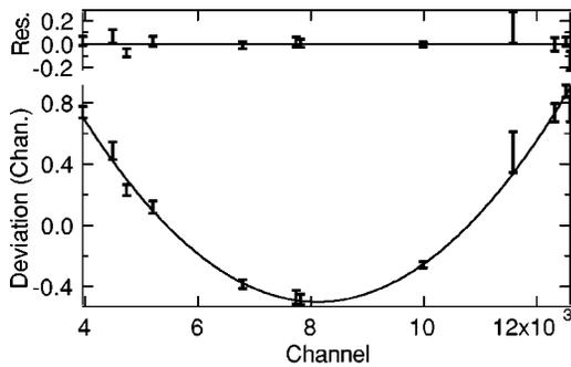
FIG. 4. Calibration of a  $\gamma$ -ray energy spectrum using the lines from  $^{56}\text{Co}$ , as described in the text. The residuals are in millichannels.
