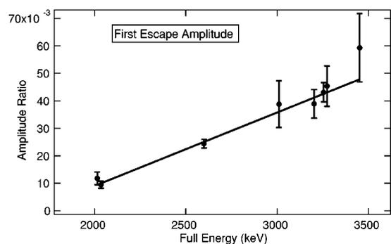
FIG. 9. The amplitudes of eight first escape peaks from  $^{56}\text{Co}$ , in terms of the amplitudes of the full energy peaks. The continuous line is the best fit to the points as a parabolic function of the full energy.
