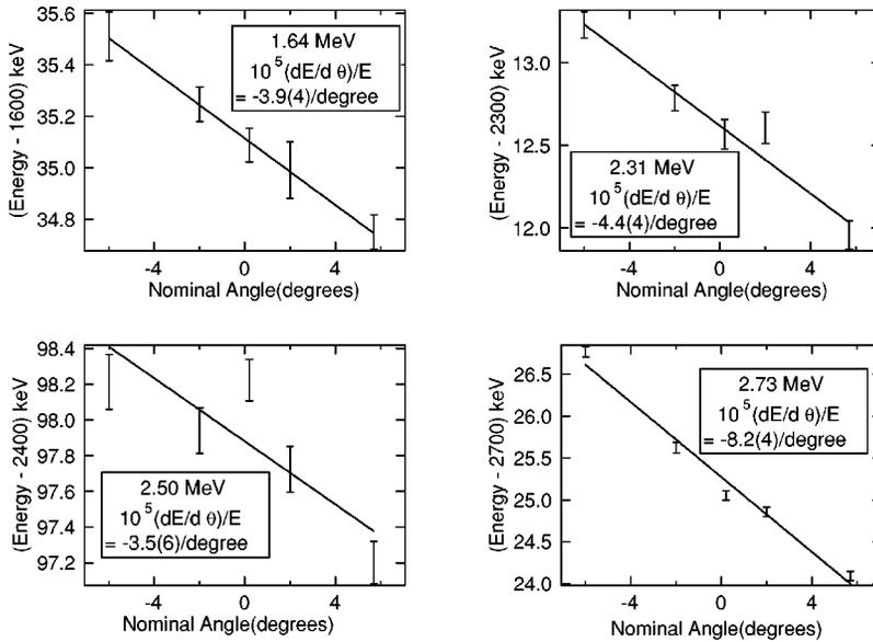
FIG. 10. The variation of observed energy of the 1.64, 2.31, 2.50, and 2.73 MeV lines from  $^{14}\text{N}$  as a function of the angle of rotation of the detection system. One nominal degree was 0.99 true degrees. (Five such sets of measurements were taken, see text.)
