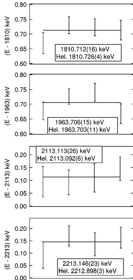
FIG. 5. Four energy determinations of four weak lines from  $^{56}\text{Co}$  which lie in the energy range of interest, and their comparison with the accepted values from Ref. [4]. The value for the 2.21 MeV line is obviously wrong.
