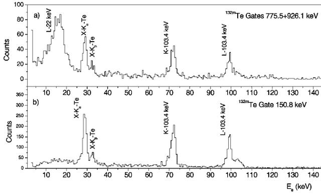
FIG. 1. Si(Li) coincidence spectra for  $^{132m}\text{Te}$  gated by  $\gamma$  rays.
