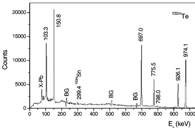
FIG. 2.  $\gamma$  ray decay of the  $^{132m}\text{Te}$  isomer. A new line of 798 keV is observed. The  $^{132m}\text{Sn}$  contaminant, previously studied [11], is very weakly produced in the present experiment.
