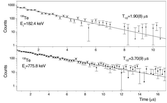
FIG. 3. Half-life spectra of the  $^{130m}\text{Te}$  and  $^{132m}\text{Te}$  isomers.
