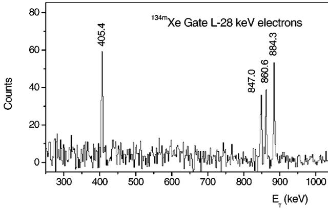
FIG. 5.  $\gamma$  spectrum of  $^{134m}\text{Xe}$  gated by the 28 keV  $L$ -electron line detected by the Si(Li) detector.
