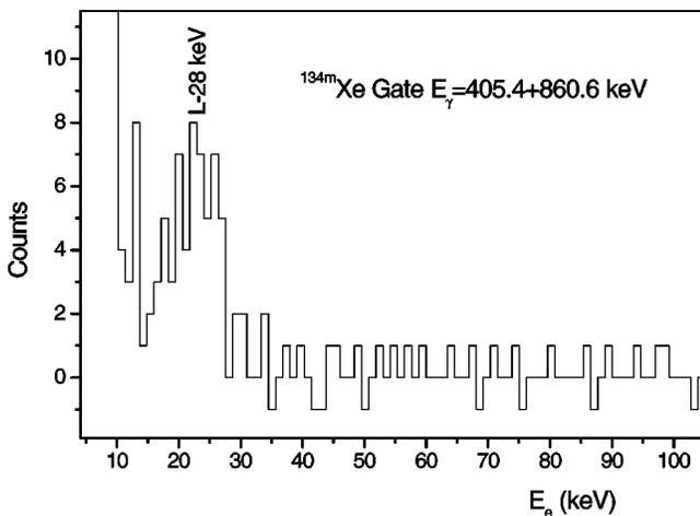
FIG. 6. Si(Li) spectrum of  $^{134m}\text{Xe}$  gated by the sum of the 405.4 and 860.6 keV  $\gamma$  rays. The 23 keV electron line observed is interpreted as the  $L$ -electron group of the 28 keV isomeric transition.
