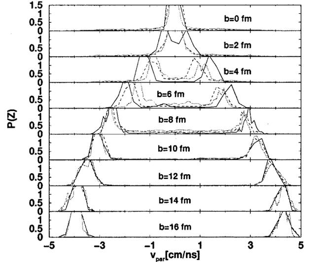
FIG. 9. The matter distribution versus velocity of Ta+Au collisions at  $E_{lab}/A=33$  MeV and different impact parameter in the BUU (solid line), nonlocal kinetic equation (dashed line) as well as the nonlocal model with quasiparticle renormalization (dotted line).
