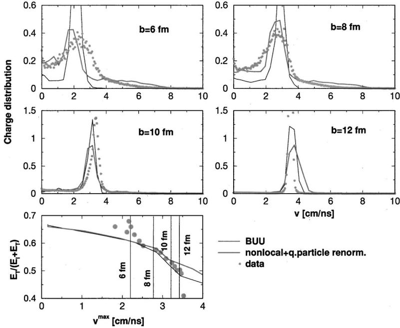
FIG. 10. The experimental charge distribution of matter (dotted line) versus velocity in comparison with the BUU (thin solid line) and the nonlocal model with quasiparticle renormalization (thick line). The maximum velocity versus ratio of longitudinal to total kinetic energy of Ta+Au collisions at  $E_{lab}/A=33$  MeV is given below. The selected experimental cuts are given by dots.
