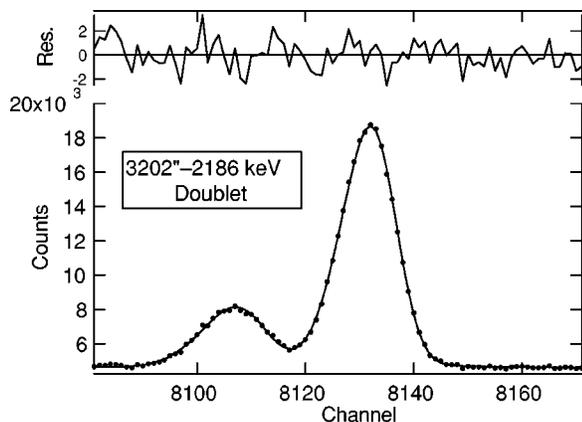
FIG. 6. The fit to the  $^{56}\text{Co}(3.202'')$ – $^{90}\text{Nb}(2.186)$  doublet using the shape of the  $^{56}\text{Co}$  2.59-MeV line. The residuals are the difference between the data and the fit, divided by the square root of the data.
