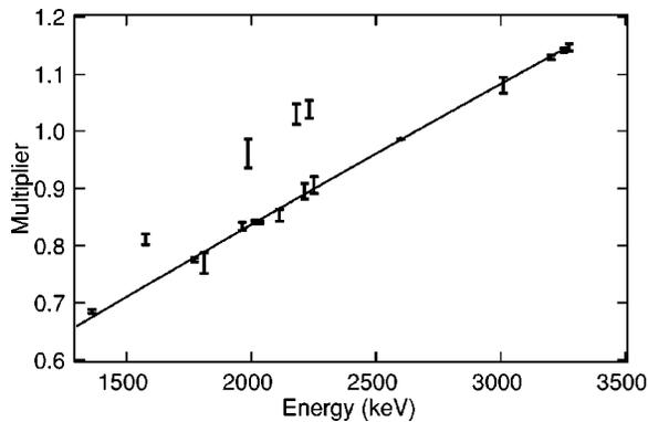
FIG. 2. The width multiplier for all the lines of  $^{56}\text{Co}$  from 1.36 to 3.27 MeV, and the fit to this in terms of a parabolic function of the line energy. The four points above the line are from second escape peaks.
