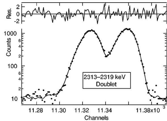
FIG. 7. The fit to the  $^{14}\text{O}(2.313)$ – $^{90}\text{Nb}(2.319)$  doublet using the shape of the  $^{56}\text{Co}$  2.59-MeV line. The residuals are the difference between the data and the fit, divided by the square root of the data.
