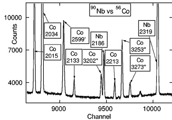
FIG. 3. Part of the energy spectrum of a mixed source of  $^{90}\text{Nb}$  and  $^{56}\text{Co}$ . The energies in keV volts are indicated, and the ' and '' designations denote single and double escape peaks, respectively.
