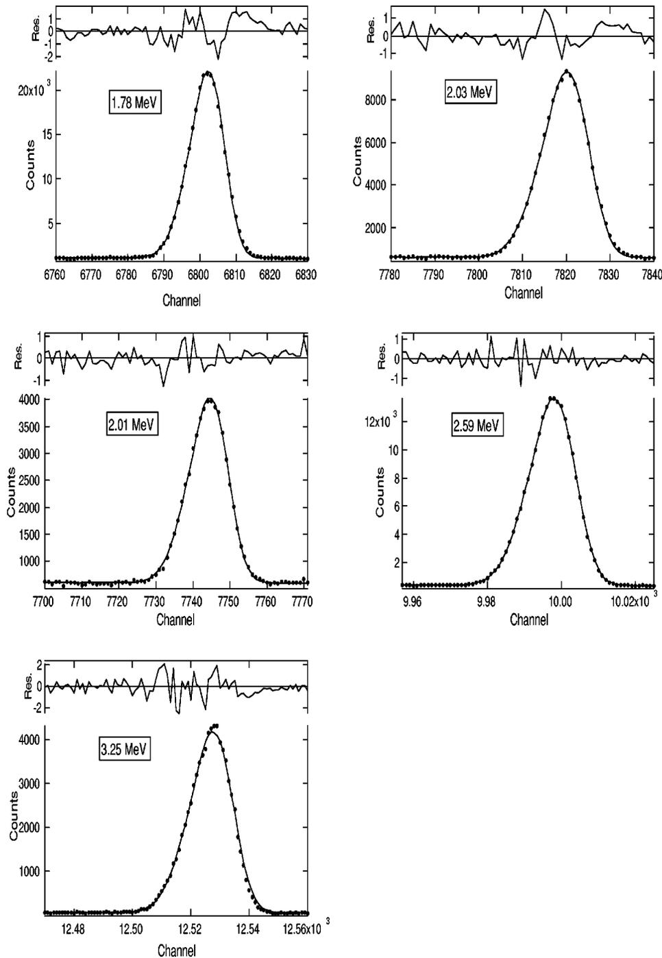
FIG. 1. Fits to the shapes of the  $^{56}\text{Co}$  lines at 1.77, 2.01, 2.03, 2.59, and 3.25 MeV, using the shape of the 2.59-MeV line, as described in the text. The residuals are the difference between the data and the fit, divided by the square root of the data.
