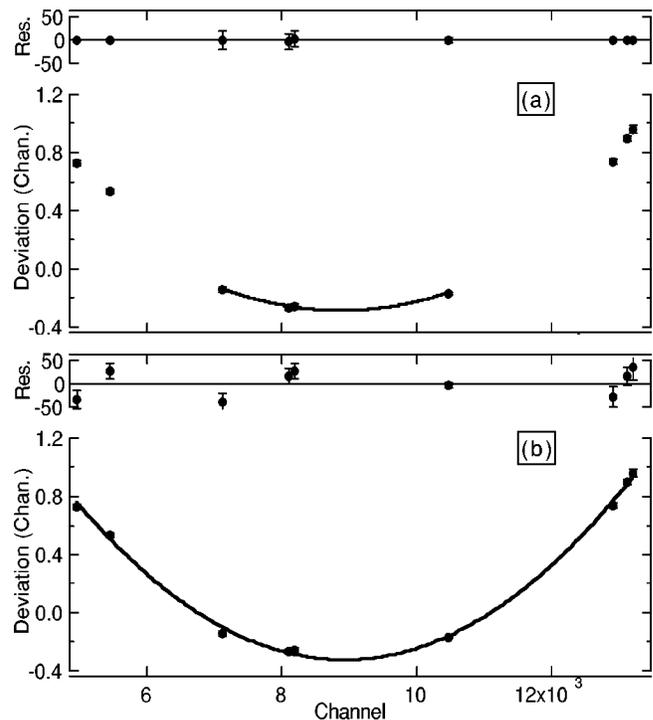
FIG. 4. Short and long calibrations of a  $\gamma$ -ray energy spectrum using the lines from  $^{56}\text{Co}$ , as described in the text. The residuals are in millichannels.
