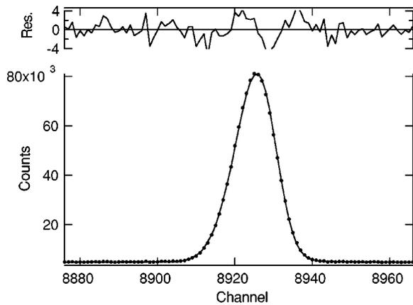
FIG. 5. The fit to the  $^{90}\text{Nb}$  2.319-MeV line using the shape of the  $^{56}\text{Co}$  2.59-MeV line. The residuals are the difference between the data and the fit, divided by the square root of the data.
