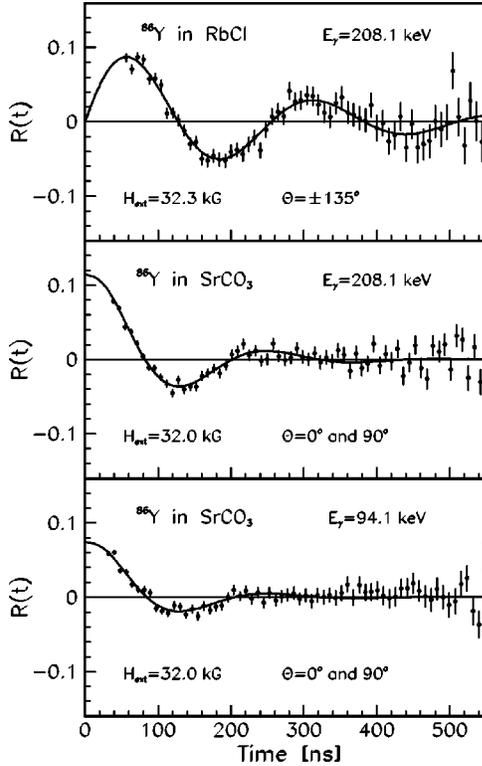
FIG. 4. TDPAD spectra of the 94.1 and 208.1 keV  $\gamma$  rays deexciting the 125 ns isomeric state in  $^{86}\text{Y}$ .
