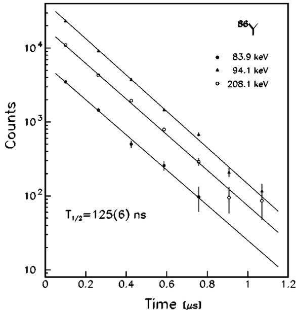
FIG. 2. Decay curves obtained from time gated energy spectra registered with the planar Ge detector.
