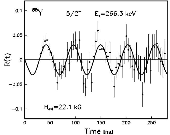
FIG. 5. TDPAD spectrum of the 266.3 keV  $\gamma$  ray deexciting the 178 ns isomeric state in  $^{85}\text{Y}$ .
