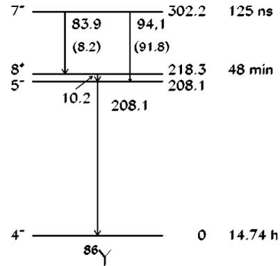
FIG. 3. Decay scheme of the 125 ns isomeric state in  $^{86}\text{Y}$ . The data concerning the  $5^-$  and  $8^+$  levels were taken from Ref. [14].
