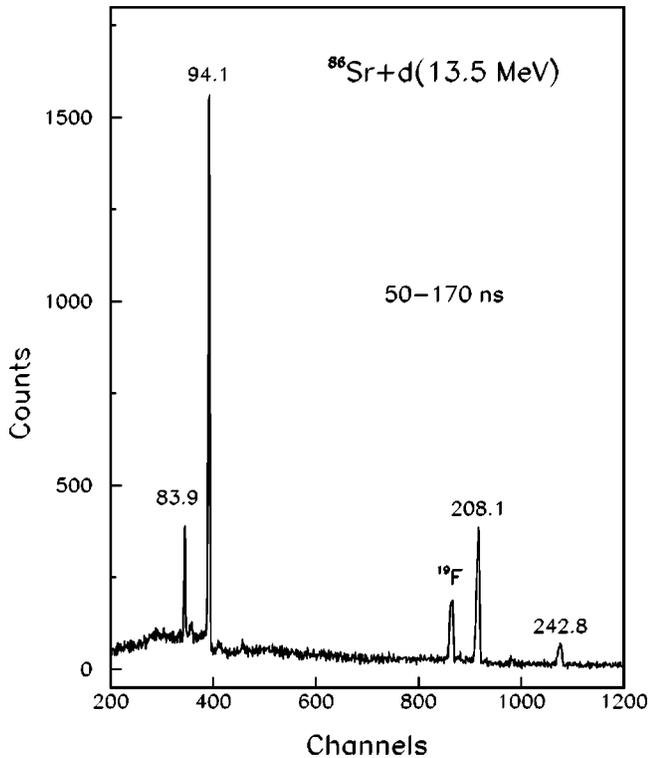
FIG. 1. Delayed spectrum corresponding to the 50–170 ns time interval. Transitions assigned to  $^{86}\text{Y}$  are labeled by energies. The 242.8 keV  $\gamma$ -ray deexcites the  $2^-$  28.5 ns isomer in  $^{86}\text{Y}$  [14].
