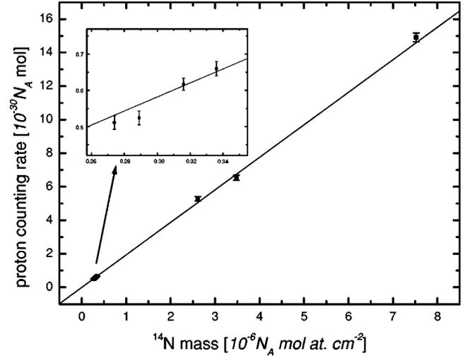
FIG. 4. A weighted linear fit through the origin for the normalized proton counting rates versus the  $^{14}\text{N}$  mass. The slope is the  $^{14}\text{N}(n_{\text{th}},p)^{14}\text{C}$  reaction cross section  $\sigma_p$ .
