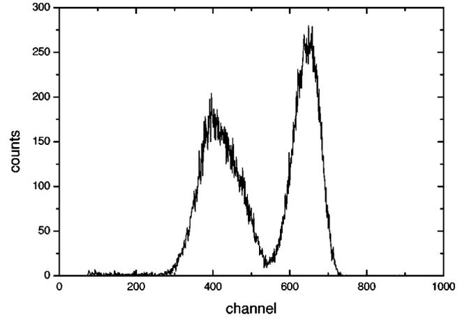
FIG. 2. Fission fragments detected during the  $^{235}\text{U}(n_{\text{th}},f)$  flux calibration.
