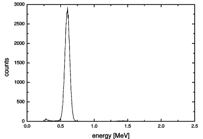
FIG. 3. Energy distribution for the  $^{14}\text{N}(n_{\text{th}},p)^{14}\text{C}$  reaction obtained with an adenine sample after 45 min of data taking.
