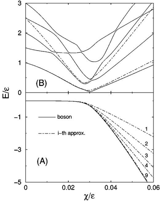
FIG. 5. Ground-state energy (A) and excitation energies of the lowest five states (B) as functions of the strength  $\chi/\epsilon$ . The solid lines are obtained by diagonalizing  $H_B$  (3) in  $B$  (4), while dot-dashed lines refer to calculations involving only the lowest Tamm-Dancoff boson and  $1p-1h$  excitations. The numbers label different orders of approximation. Further details in Sec. V.
