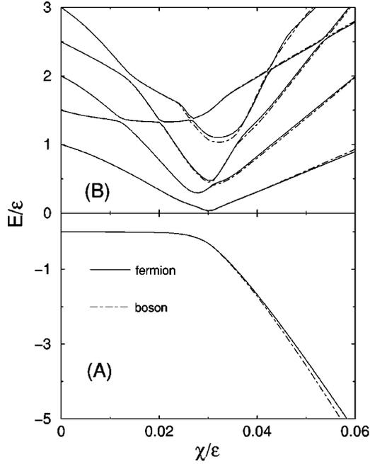
FIG. 1. Ground-state energy (A) and excitation energies of the lowest five states (B) as functions of the strength  $\chi/\epsilon$ . The solid lines are obtained by diagonalizing  $H_F$  (3) in  $F$  (4), while dot-dashed lines refer to  $H_B$  (7) in  $B$  (5).
