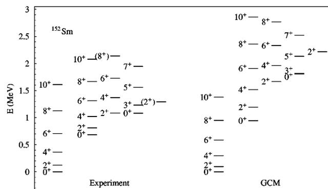
FIG. 1. Energy levels of  $^{152}\text{Sm}$ . Left, experiment; right, GCM calculations discussed in the text.
