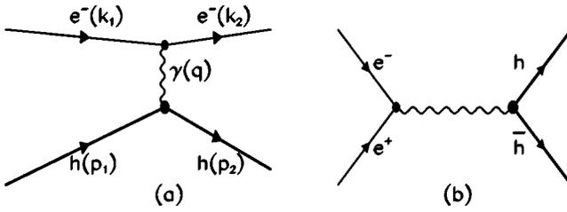
FIG. 1. One-photon approximation for the crossed channels  $e^- + h \rightarrow e^- + h$  and  $e^- + e^+ \rightarrow h + \bar{h}$ .
