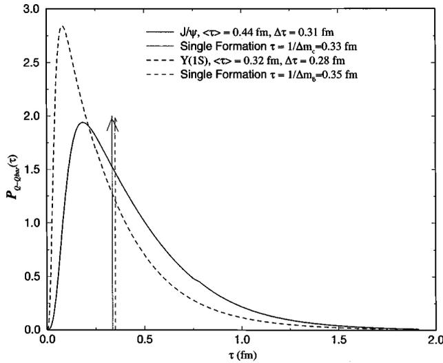
FIG. 2. Normalized distribution functions for formation times of  $J/\psi$  and  $Y$  in  $e^+e^-$  annihilation.
