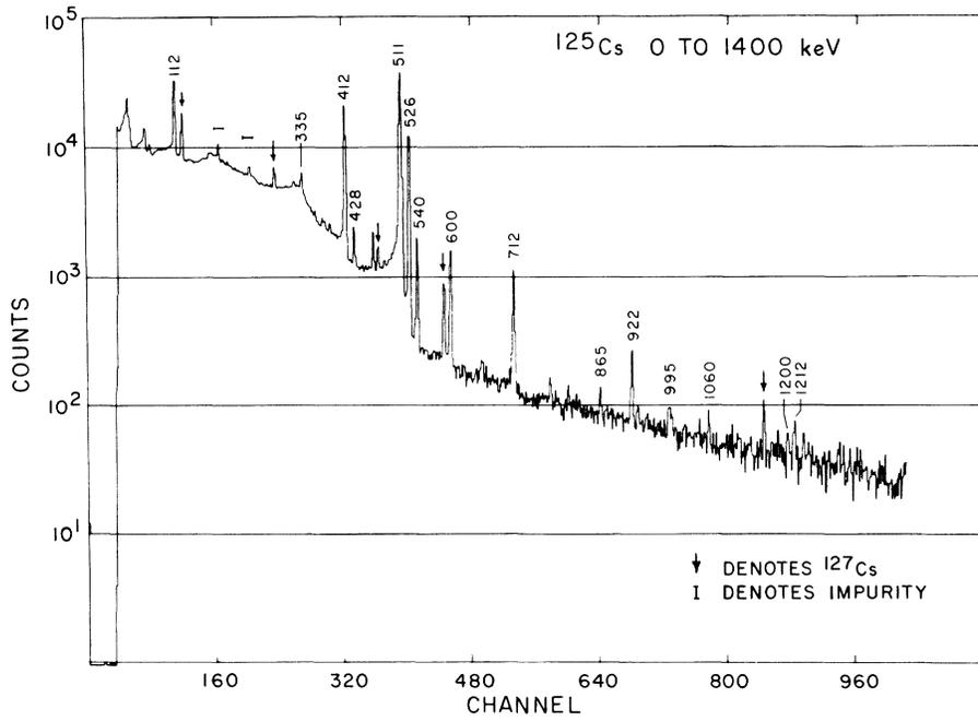
FIG. 6.  $\gamma$ -ray spectrum of  $^{125}\text{Cs}$  (low-energy portion). Some of these  $\gamma$  rays have been observed by W. R. Kane, *Bull. Am. Phys. Soc.* 16, 551 (1971).
