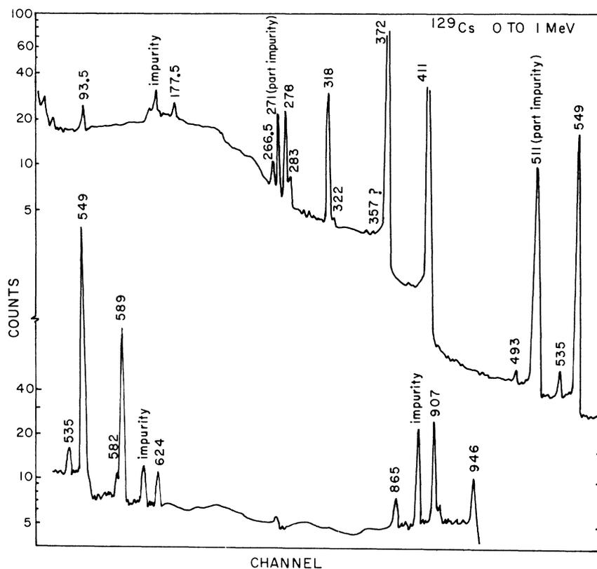
FIG. 1.  $\gamma$ -ray spectrum of  $^{129}\text{Cs}$ .
