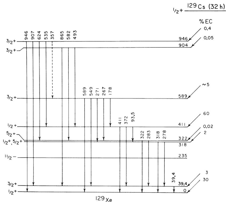
FIG. 2. Decay scheme of  $^{129}\text{Cs}$ .
