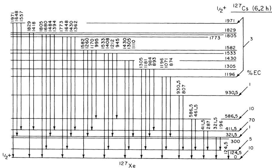
FIG. 5. Decay scheme of  $^{127}\text{Cs}$ .
