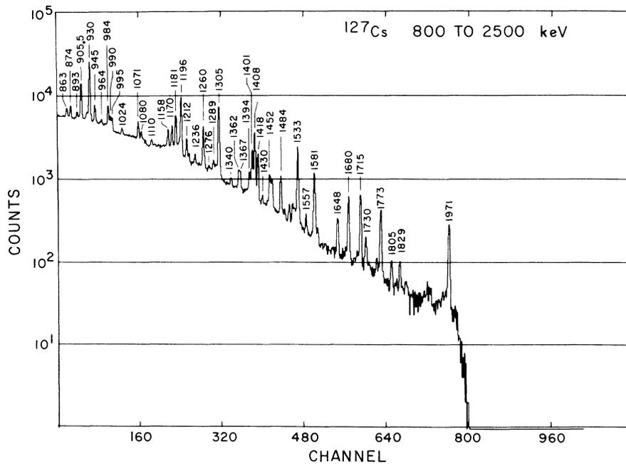
FIG. 4.  $\gamma$ -ray spectrum of  $^{127}\text{Cs}$  up to 2800 keV.
