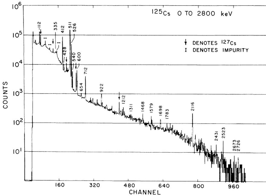
FIG. 7.  $\gamma$ -ray spectrum of  $^{125}\text{Cs}$  (from 100 to 3000 keV).
