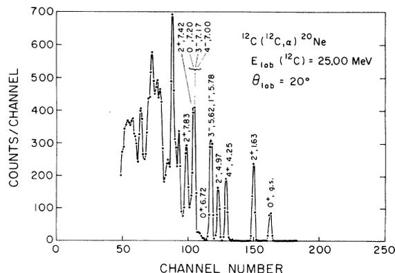
FIG. 1.  $\alpha$  spectrum obtained at  $20^\circ$  for the  $^{12}\text{C}(^{12}\text{C}, \alpha)^{20}\text{Ne}$  reaction at 25.0 MeV.
