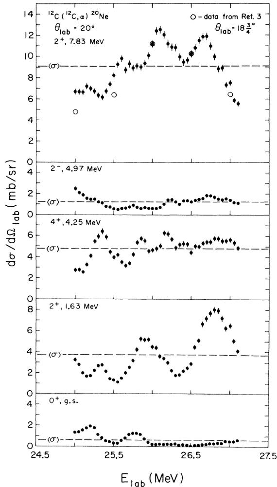
FIG. 2. Excitation functions measured at  $20^\circ$  (lab) for the  $^{12}\text{C}(^{12}\text{C}, \alpha)^{20}\text{Ne}$  reaction at low-lying states.
