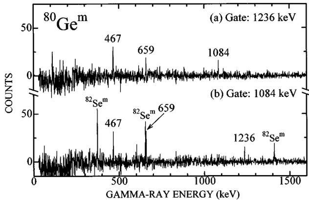
FIG. 2. Coincidence spectra of  $\gamma$  rays from the  $^{80}\text{Ge}^m$  isomer. The gates were set on the  $\gamma$  rays with energies of (a) 1236 and (b) 1084 keV.
