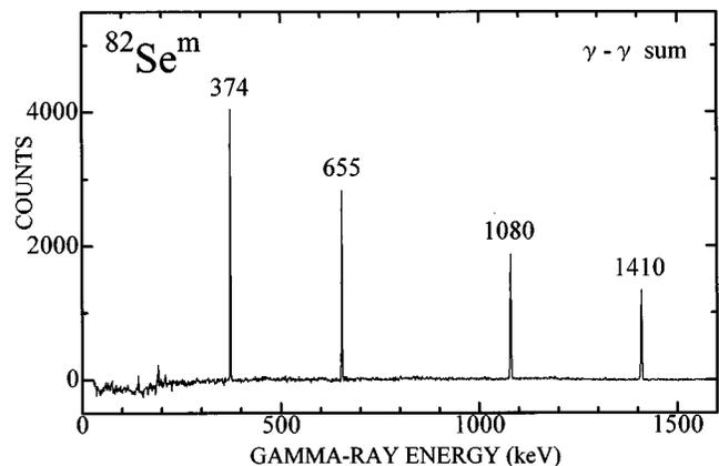
FIG. 1. A mutual coincidence spectrum of  $\gamma$  rays from the new  $^{82}\text{Se}$  isomer. The gates for sorting the event records were set on the 374, 655, 1080, and 1410 keV  $\gamma$  rays.
