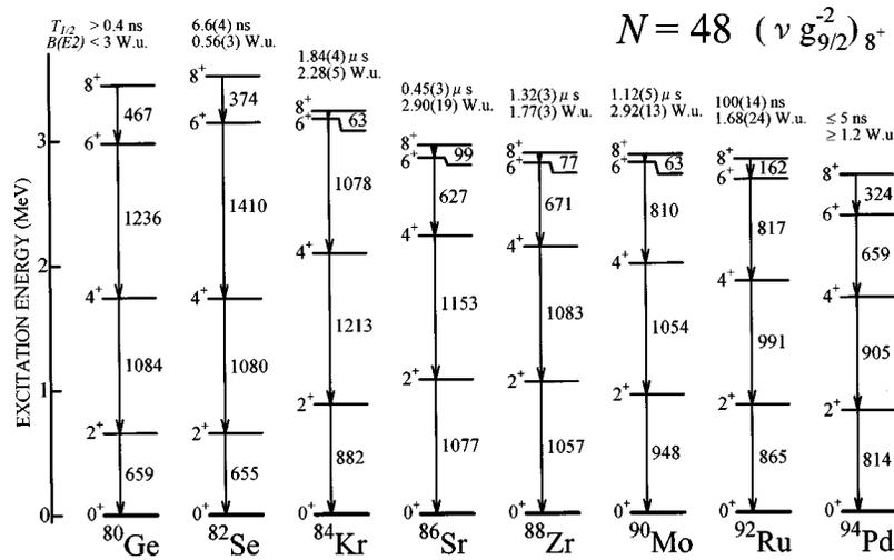
FIG. 4. Decay schemes of the  $8^+$  isomers in the  $N=48$  isotones from  $^{80}_{32}\text{Ge}$  to  $^{94}_{46}\text{Pd}$ . Transition energies are given in units of keV. The  $B(E2; 8^+ \rightarrow 6^+)$  values are also shown.
