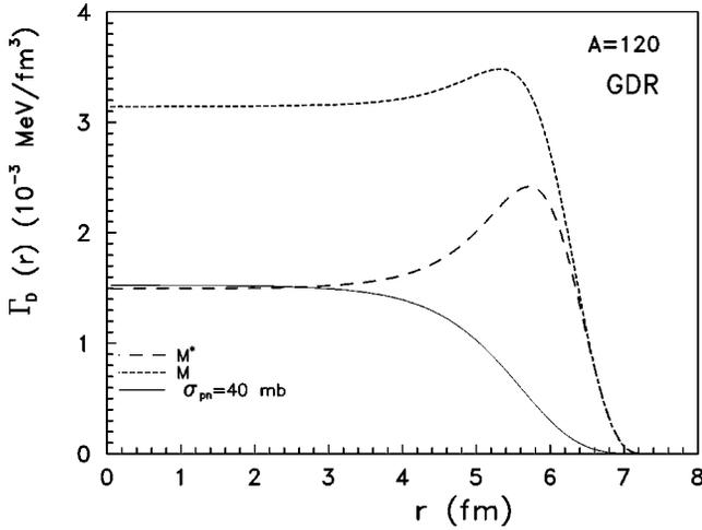
FIG. 1. The relative contribution to the collisional damping width of GDR as a function of  $r$  for  $A=120$  at zero temperature. Solid, dashed, and dotted lines are calculations with a constant cross section  $\sigma_{pn}=40$  mb, with the SkM force with the effective mass, and with the SkM force with the bare mass, respectively.
