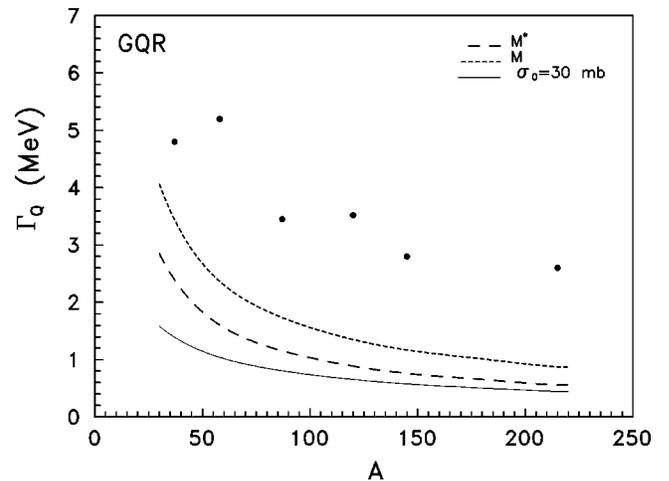
FIG. 4. The collisional damping width of GQR as a function of mass number  $A$  at zero temperature. Solid, dashed, and dotted lines are calculations with a constant cross section  $\sigma_{pn}=30$  mb, with the SkM force with the effective mass, with the SkM force with the bare mass, respectively, and the points show the data.
