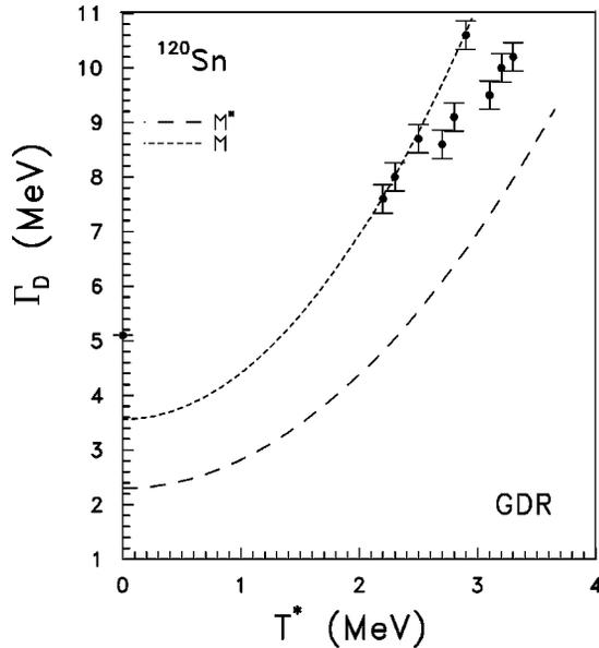
FIG. 5. The collisional damping width of GDR in  $^{120}\text{Sn}$  as a function of temperature. Dashed, dotted lines, and points are calculations with the SkM force with the effective mass, with the SkM force with the bare mass, and data taken from [2], respectively.
