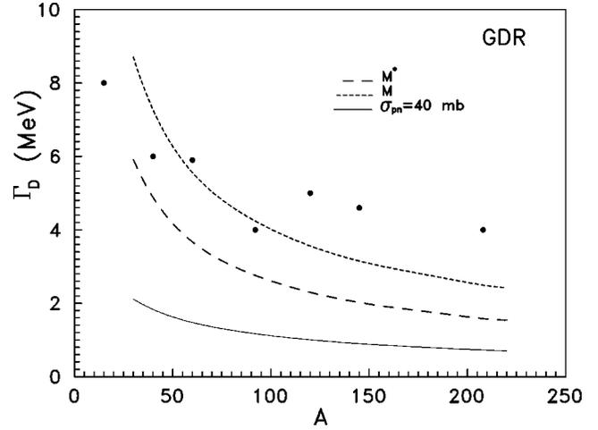
FIG. 3. The collisional damping width of GDR as a function of mass number  $A$  at zero temperature. Solid, dashed, and dotted lines are calculations with a constant cross section  $\sigma_{pn}=40$  mb, with the SkM force with the effective mass, with the SkM force with the bare mass, respectively, and the points show the data.
