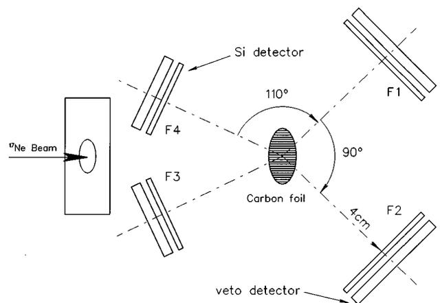
FIG. 2. Detector arrangement for the detection of  $p\text{-}\alpha\text{-}^{12}\text{C}$  triple coincidences from the decay of the IAS in  $^{17}\text{F}$ .
