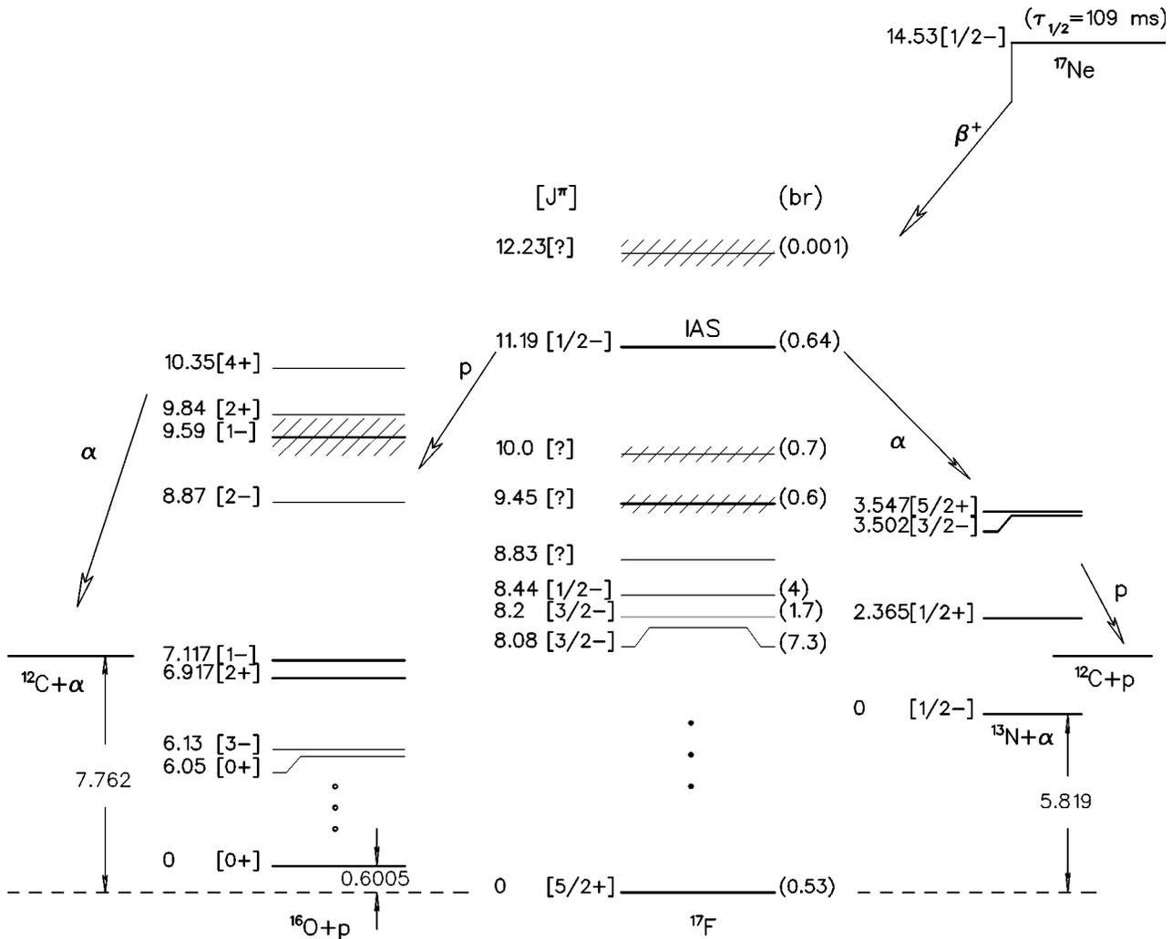
FIG. 1. Partial decay scheme of  $^{17}\text{Ne}$  [2,8]. States below 8 MeV in  $^{17}\text{F}$  are omitted since they cannot populate the  $2^+$  state at 6.917 MeV in  $^{16}\text{O}$  via proton decay.
