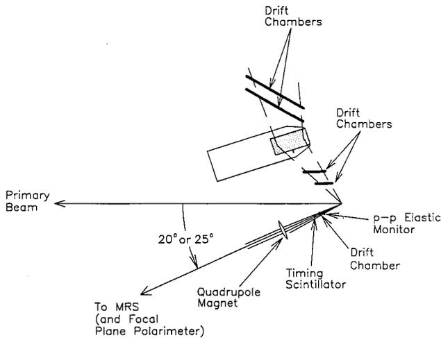
FIG. 1. Experimental setup for the  $^{16}\text{O}(p,2p)$  experiment. The high-energy proton was detected in the medium resolution spectrometer (MRS) which is only partially shown, and the low-energy proton was detected by the nonfocusing magnetic spectrometer on the other side of the beamline.
