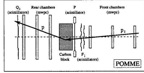
FIG. 4. Polarimeter POMME: The hodoscope of plastic scintillators  $F_i$  is located at the final focalization (FF) of the spectrometer. The  $P$  and  $Q_i$  lath of plastic scintillators are connected to photomultipliers on each side.
