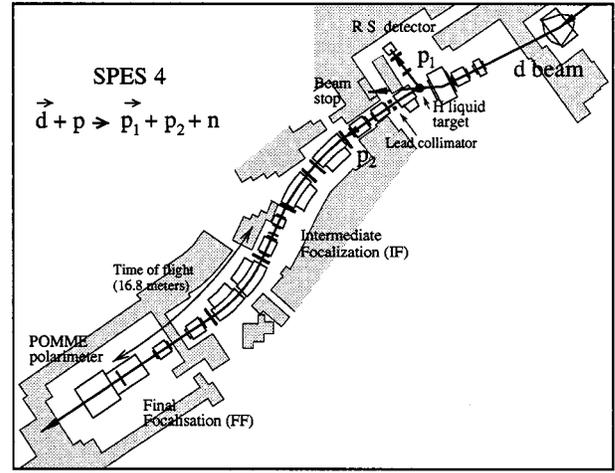
FIG. 3. Experimental setup: The magnets of the beam line and of the SPES 4 spectrometer are shown with the location of the RS arm and of the POMME polarimeter. The shaded areas are concrete walls. The RS detectors are protected from a direct view of the beam stop.
