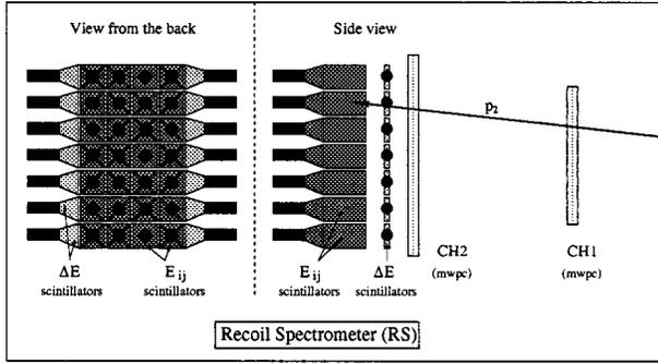
FIG. 5. Recoil Spectrometer (RS): The RS arm is shown from the side (on the right part) and from the back (on the left part). The distance between  $E_{ij}$  scintillators and between  $\Delta E$  scintillators is enlarged on the picture. The distance is actually only the wrapping papers.
