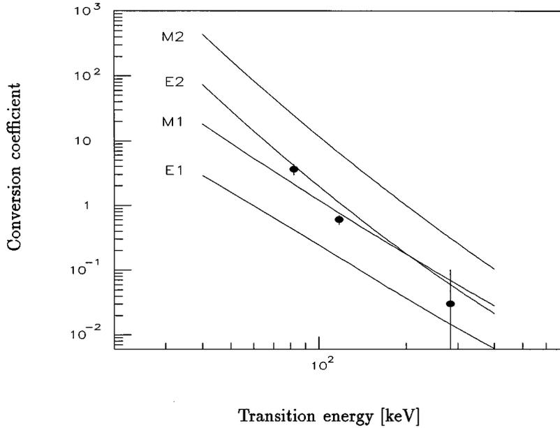
FIG. 2. Experimental and theoretical total internal conversion coefficients for the three lowest transitions in the  $^{147}\text{Ce}$   $\gamma$  cascade. The theoretical values are from the tables of Röseler *et al.* [18]. Experimental values are deduced from intensity balance measurements.
