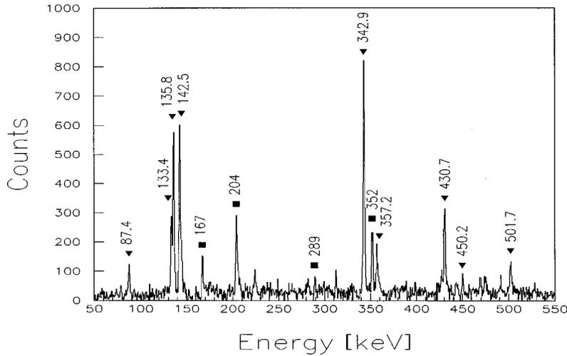
FIG. 4. Spectrum of  $\gamma$  rays in coincidence with gates set simultaneously on the 141 and 241 keV  $\gamma$  lines. Transitions in  $^{149}\text{Ce}$  are marked by full triangles and  $\gamma$  rays corresponding to complementary Sr fragments by full rectangles.
