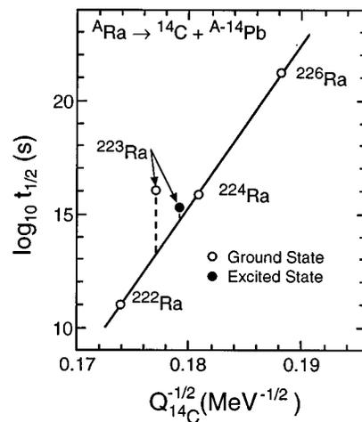
FIG. 1. Geiger-Nuttal diagram of the  $^{14}\text{C}$  radioactive decay of Ra isotopes. The logarithm of the experimental half-lives in seconds is plotted against  $Q^{-1/2}$  with  $Q$  being energy of the decay in MeV. The distance the  $^{223}\text{Ra}$  points are above the straight line through the even-even Ra isotopes is used to determine the hindrance factors.
