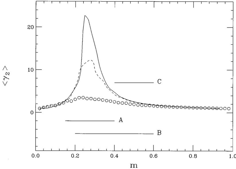
FIG. 1. Reduced variance  $\langle \gamma_2(m) \rangle$  as a function of the reduced multiplicity  $m$  calculated within the bond percolation model with  $6^3$  (circles),  $15^3$  (dashed line), and  $20^3$  (solid line) sites. Brackets reproduce the  $m$ -gating intervals for “near-critical” events used in this work (bracket A) and in the original study of Ref. [3] (bracket B). The “optimal range” of  $m$  gating for the appearance of intermittency is also indicated (bracket C).
