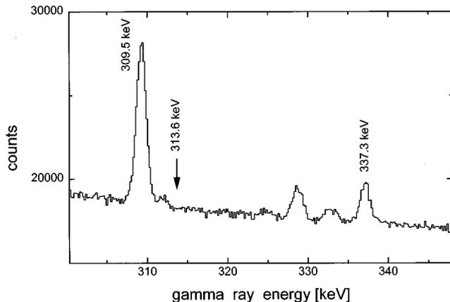
FIG. 3.  $\gamma$ -ray spectrum observed in the decay of 29 h  $^{160}\text{Er}$ . The energy resolution in the region shown in the figure was full width at half maximum (FWHM)  $\sim 1.4$  keV.
