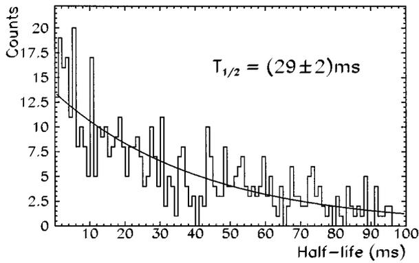
FIG. 2. Decay-time characteristics for the proton groups between 1.8 MeV and 2.4 MeV of  $^{22}\text{Si}$ . The solid line is a maximum likelihood fit with a single decay component plus a daughter decay yielding a half-life of  $T_{1/2} = (29 \pm 2)$  ms.
