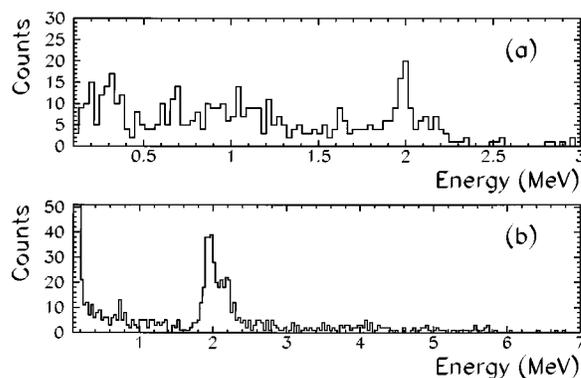
FIG. 1. Charged-particle spectra measured after implantation of a  $^{22}\text{Si}$  isotope in the MSGC (a) and in the silicon detector (b). Energies and branching ratios are given in the text.
