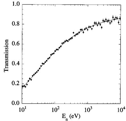
FIG. 2. Neutron transmission through 0.277 g/cm<sup>2</sup> of the boron powder. The solid curve is the result of a fit to the data assuming the functional form given in Eq. (2).
