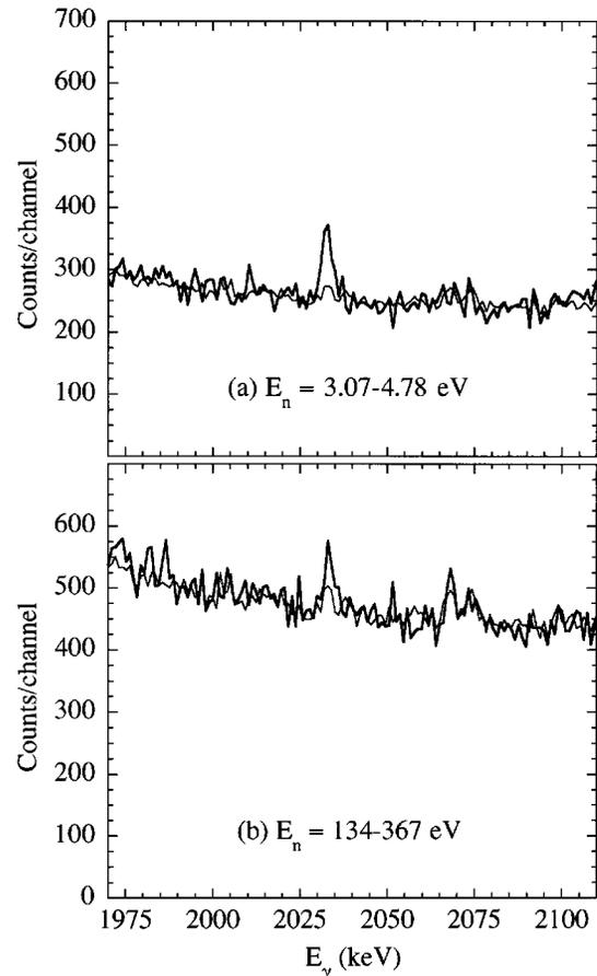
FIG. 3. Gamma-ray energy spectrum showing the region around  $E_\gamma = 2033 \text{ keV}$ . The heavy line is the raw spectrum taken with the  ${}^7\text{Li}$  target. The light line is the background data collected with the scattering sample, which have been normalized to the  ${}^7\text{Li}$  data outside the region of the 2033-keV peak.
