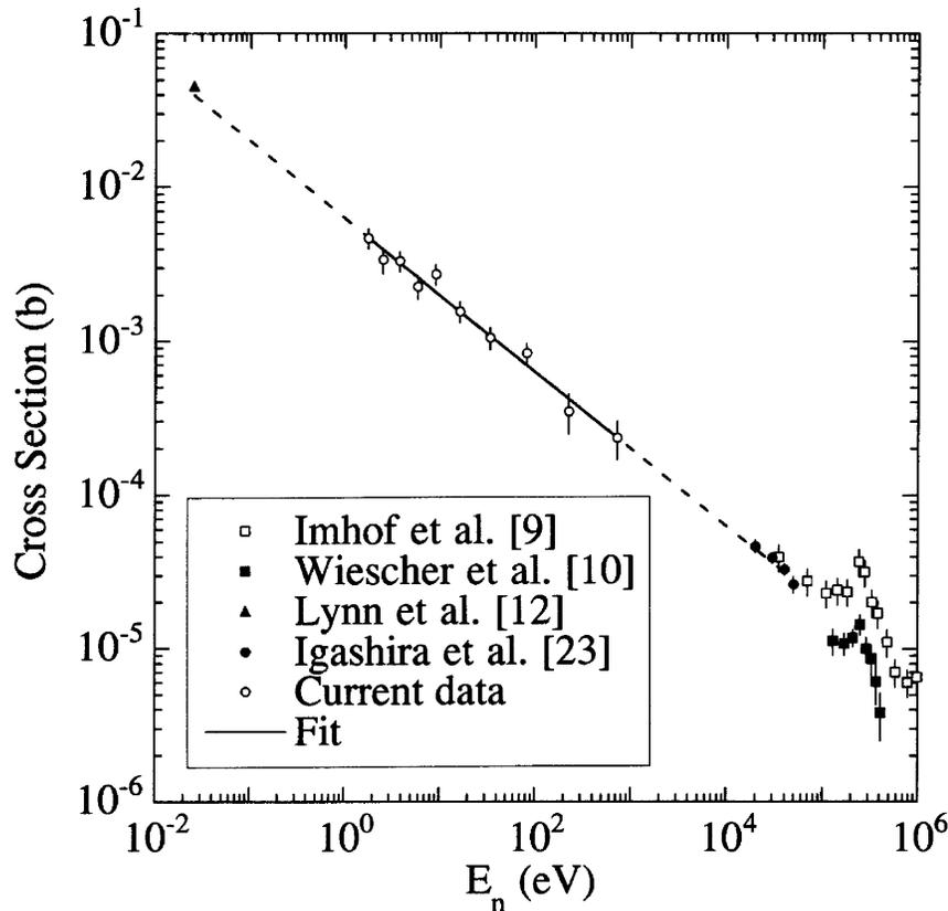
FIG. 4. Measurements of cross sections for the  ${}^7\text{Li}(n, \gamma){}^8\text{Li}$  capture reaction. The solid line is a  $1/v$  fit to the data from the current measurement.
