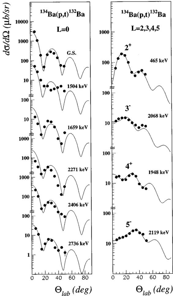
FIG. 1. Angular distributions of the cross sections for  $^{134}\text{Ba}(p,t)^{132}\text{Ba}$  with DWBA calculations. At the left side  $L=0$  transitions for the lowest six  $0^+$  states and at the right side selected  $L=2,3,4,5$  transitions. Note the changes in the scales. For the DW calculations the code TWOFNR, with standard optical model parameters has been used.
