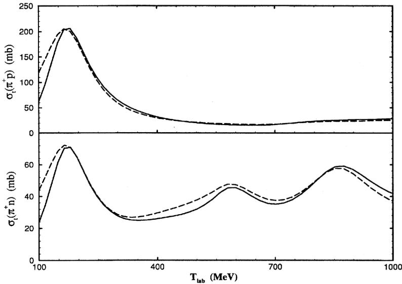
FIG. 2. Total cross sections for pion-nucleon scattering. The solid line is the result of the phase shift analysis of Arndt. The dashed line replaces the  $\Delta_{33}(1232)$ , the  $D_{13}(1520)$ , and the  $F_{15}(1680)$  channels by the Breit-Wigner form with parameters as taken from Kondratyuk *et al.*
