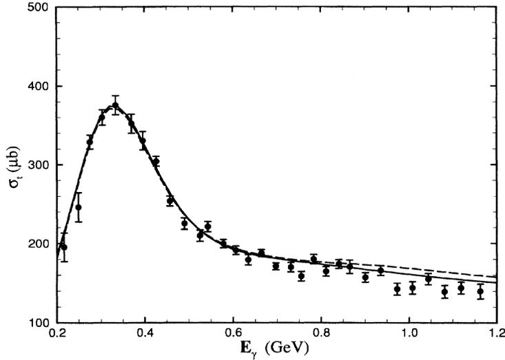
FIG. 1. The total cross section for photon- $^{238}\text{U}$  scattering as a function of photon energy. The data are from Kondratyuk *et al.* The solid line is the result of the model presented there where eight resonances have enhanced widths. The dashed line is the result of their model with only three resonances having medium modified widths.
