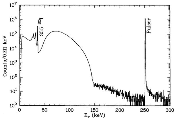
FIG. 1. A 12 hour raw spectrum of the  $^{125}\text{I}$  source recorded in a planar Ge detector.
