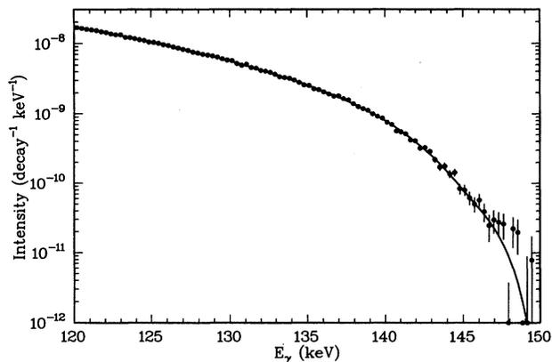
FIG. 2. Net IB spectrum of  $^{125}\text{I}$  above the  $1s$  end point. The solid line is a normalized fit using the Surić *et al.* calculation. The (multiplicative) normalization factor for the theoretical calculation is  $0.86 \pm 0.10$ .
