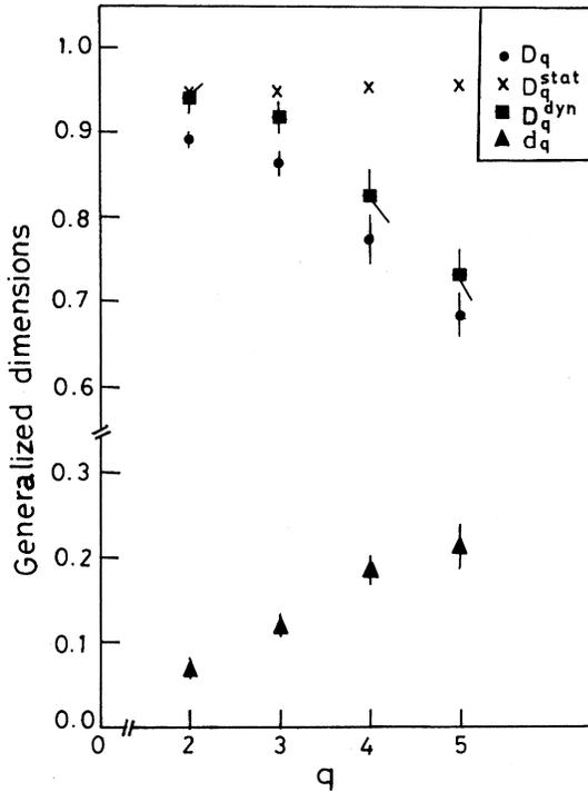
FIG. 2. Generalized dimensions  $D_q$ ,  $D_q^{\text{stat}}$ ,  $D_q^{\text{dyn}}$ , and the anomalous fractal dimension  $d_q$  as a function of order  $q$ .
