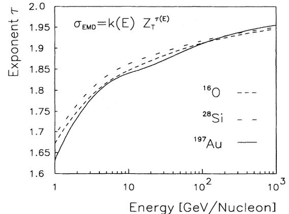
FIG. 6. Energy dependence of the exponent  $\tau$  of a power law fit  $\sigma_{\text{ED}} = k(E) Z_T^{\tau(E)}$  to the calculated charge-changing ED cross section for  $^{16}\text{O}$ ,  $^{28}\text{Si}$ , and  $^{197}\text{Au}$ .
