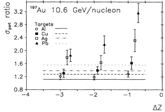
FIG. 5. Cross section ratios for targets Al/C, Cu/C, Ag/C, and Pb/C for three partial cross sections from this work. The horizontal lines show the square roots of the total charge-changing cross sections of this work.
