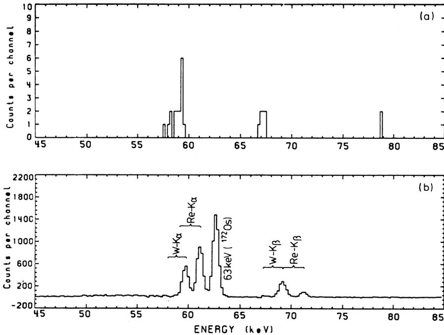
FIG. 3. (a) X and  $\gamma$  rays in coincidence with 5.166 MeV  $\alpha$  rays in  $^{171}\text{Os}$  decay measured in 48 h [sum of spectra OS2-OS6 (cf. Table I)]. (b) Total projection of  $\gamma$  ray coincidences measured in 4 h, experiment OS4.
