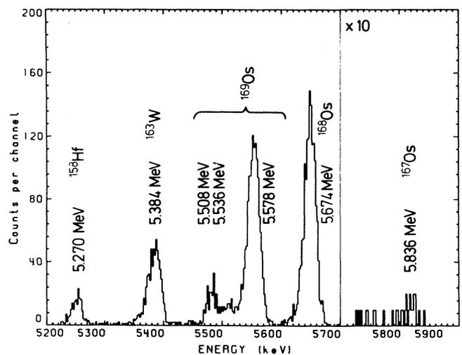
FIG. 1. Alpha spectrum of osmium isotopes observed in the reaction  $^{58}\text{Ni}+^{114}\text{Cd}$ . The beam energy in the target was 212–267 MeV, the cycle time was 8 s, and the total measurement time was 33 h.
