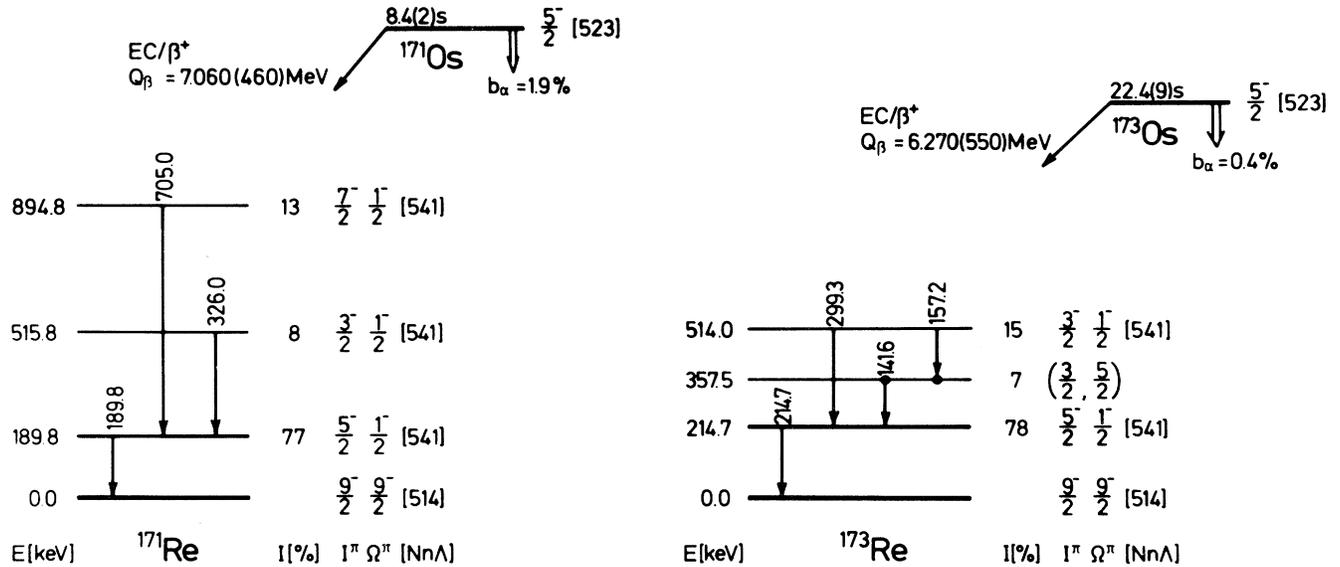
FIG. 4. Beta decay schemes of  $^{171,173}\text{Os}$ . The systematic  $Q$  values are taken from Ref. [44]. The  $\alpha$ -decay branch of  $^{171}\text{Os}$  is shown in Fig. 2.
