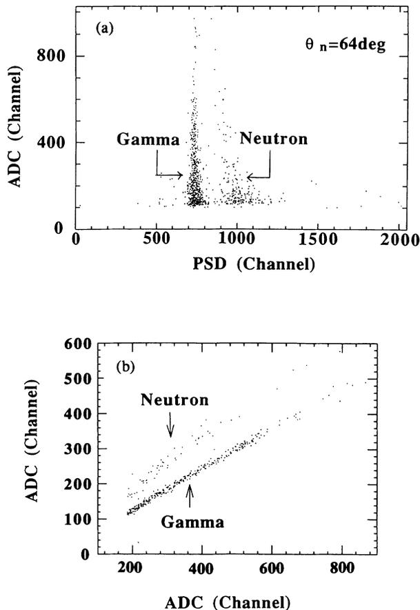
FIG. 3. (a) The two-dimensional plots of PSD-ADC signals from the neutron detector. (b) The two-dimensional plots of ADC-ADC signals from the neutron detector (charge comparison method).
