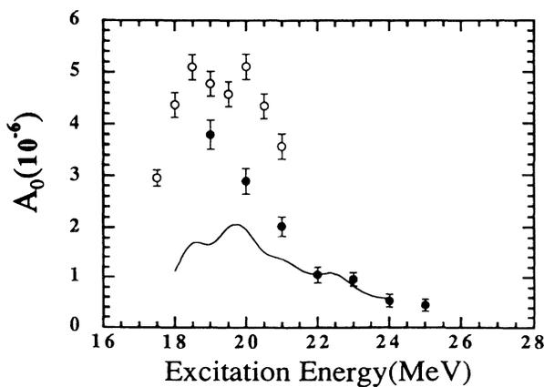
FIG. 14.  $^{40}\text{Ca}(e, e'n_0)^{39}\text{Ca}$  longitudinal and transverse cross section measured in the present work (solid circles) in comparison with that for the reaction  $^{40}\text{Ca}(e, e'p_0)^{39}\text{K}$  of Tanaka *et al.* [13] (open circles) and the values transformed from the reaction  $^{40}\text{Ca}(\gamma, n_0)^{39}\text{Ca}$  of Kellie *et al.* [4] (solid line). Same units as Fig. 13.
