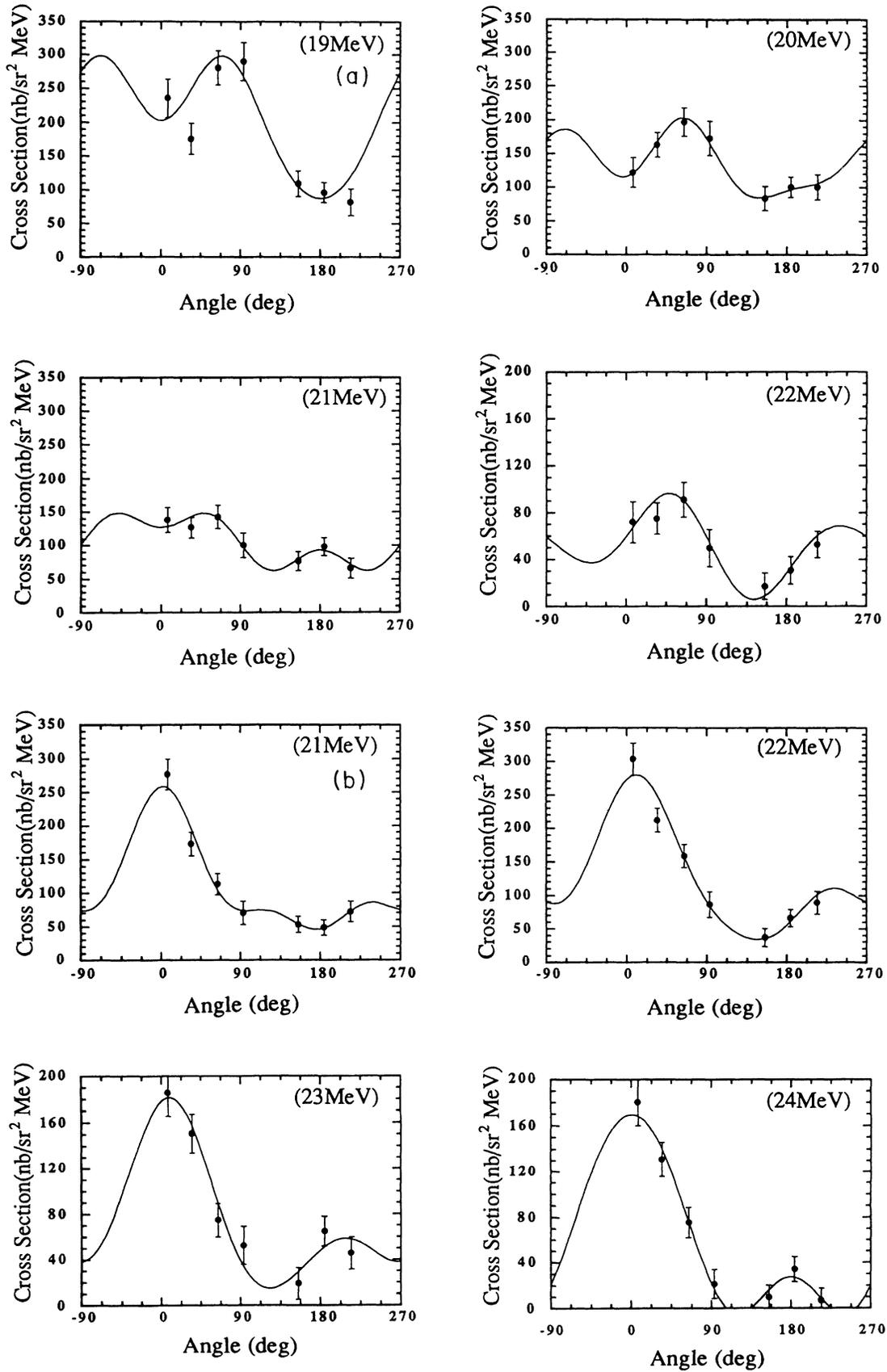
FIG. 7. Angular distributions of neutrons measured in the reactions (a)  $^{40}\text{Ca}(e, e'n_0)^{39}\text{Ca}$  and (b)  $^{40}\text{Ca}(e, e'n_1)^{39}\text{Ca}$ . The excitation energy range is indicated. Solid lines represent Legendre polynomial fits with Eq. (6).
