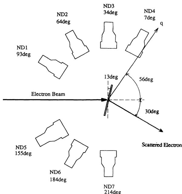
FIG. 1. Experimental arrangement. Each detector was placed 75 cm from the center of the scattering chamber. Detector angles are measured from the momentum transfer direction. An arrow indicated by  $q$  shows the direction of the momentum transfer.
