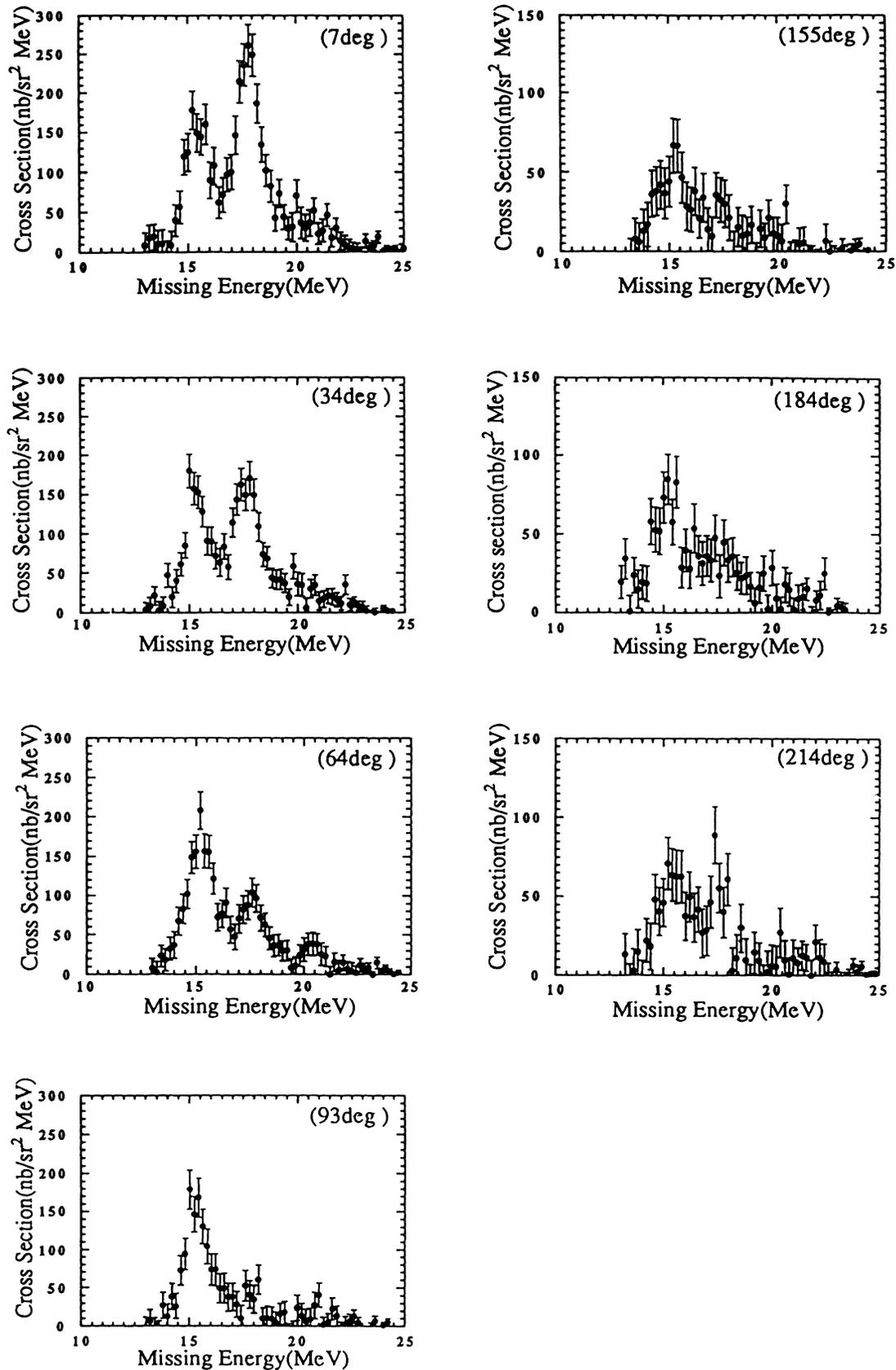
FIG. 5. Missing energy spectra for the  $^{40}\text{Ca}(e, e'n)^{39}\text{Ca}$  reaction. The peak at 15.6 MeV corresponds to the neutrons feeding the ground state in  $^{39}\text{Ca}$  and the peak at 17.8 MeV corresponds to the neutrons feeding the first, second, and third excited states in  $^{39}\text{Ca}$ .
