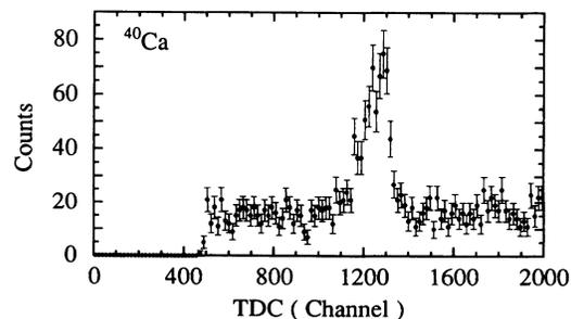
FIG. 4. Typical neutron time-of-flight spectrum. The peak is due to true events and counts in other area are accidental coincidence events.
