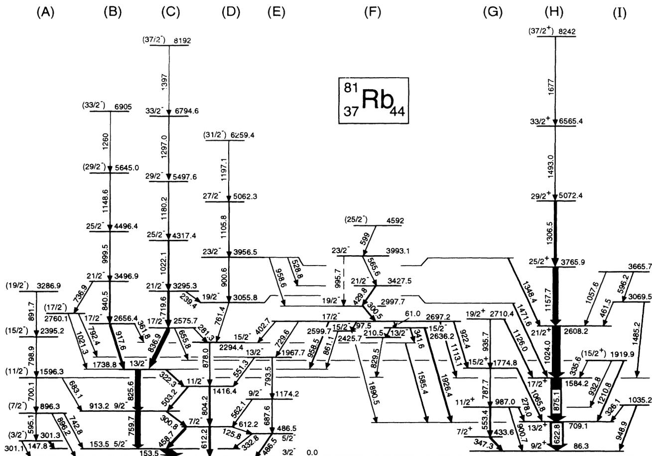
FIG. 4. Level scheme of  $^{81}\text{Rb}$  as inferred from the present data.
