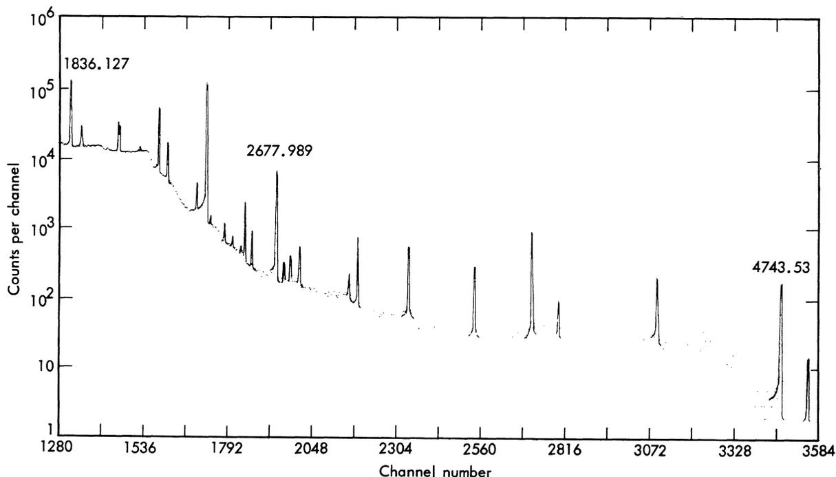
FIG. 2.  $\gamma$ -ray spectrum of the high-energy region for  $^{88}\text{Rb}$  decay taken with an LLL 40-cm<sup>3</sup> Ge(Li) detector.
