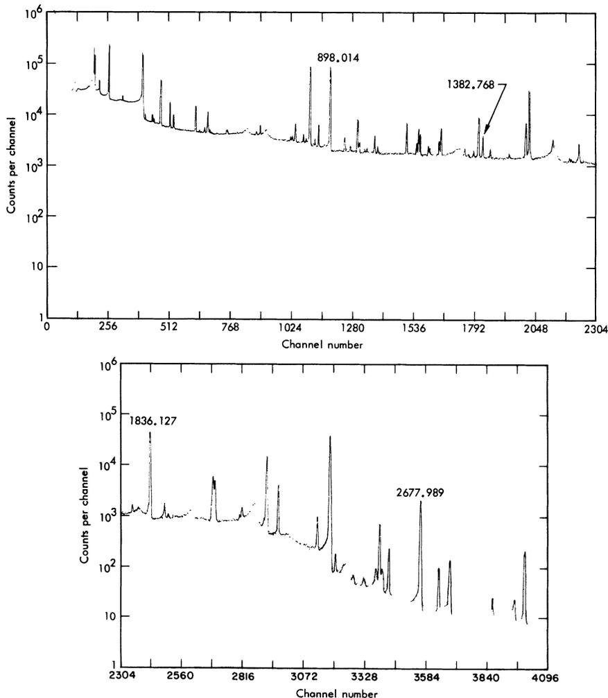
FIG. 1.  $\gamma$ -ray spectrum of a source of  $^{88}\text{Rb}$  and  $^{88}\text{Kr}$  taken with the LLL Compton-suppression Ge(Li) spectrometer.
