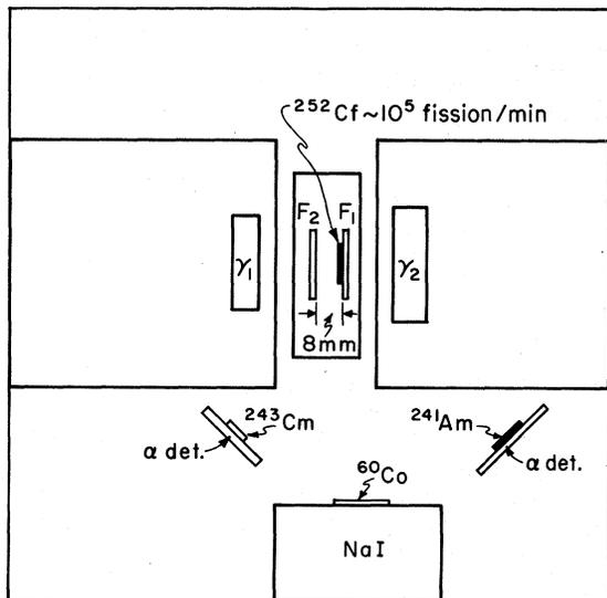
FIG. 1. Schematic representation of the experimental detector configuration. Detectors  $F_1$  (with electrodeposited  $^{252}\text{Cf}$ ) and  $F_2$  were used to measure the fragment kinetic energies. Detectors  $\gamma_1$  and  $\gamma_2$  measured energies of  $\gamma$  rays and/or x rays. The sources and detectors indicated at the bottom of the figure were used for external stabilization of the photon detectors.
