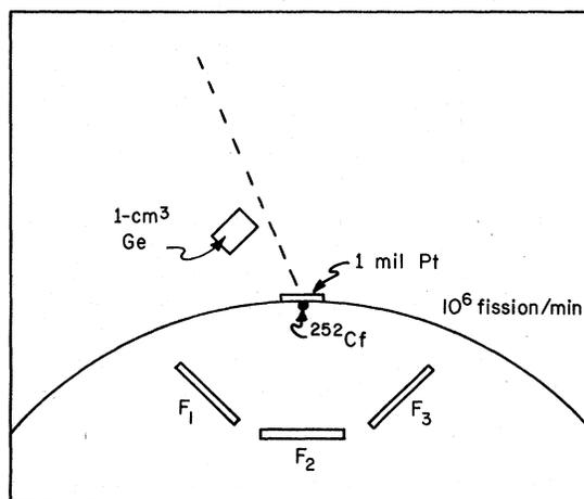
FIG. 2. Experimental configuration for the angular distribution studies of the prompt-fission  $\gamma$  rays. The dashed line is the second location of the Ge detector which allowed the angular distribution to be studied at six angles.
