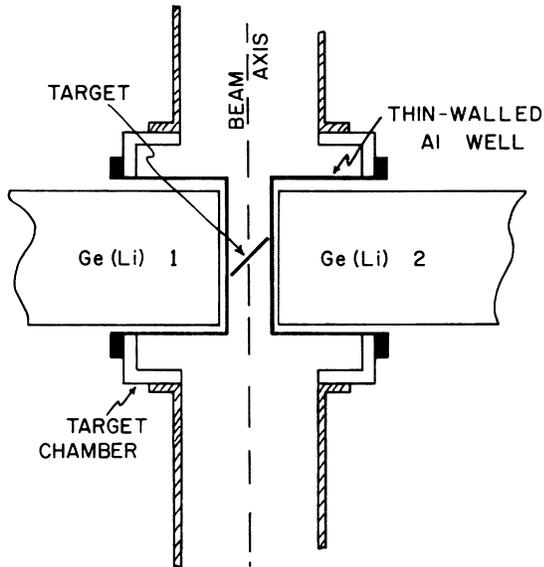
FIG. 2. Schematic diagram of the experimental arrangement for doing in-beam  $\gamma$ - $\gamma$  coincidence with two Ge(Li) detectors.
