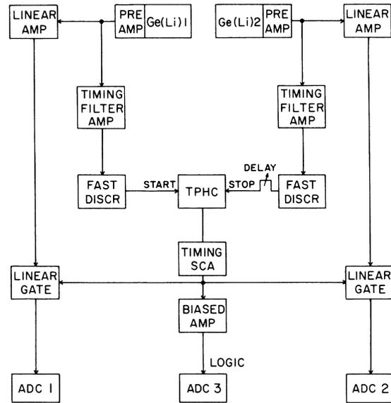
FIG. 3. Schematic of the fast-slow coincidence electronics used in the  $(p, n\gamma)$  experiment.
