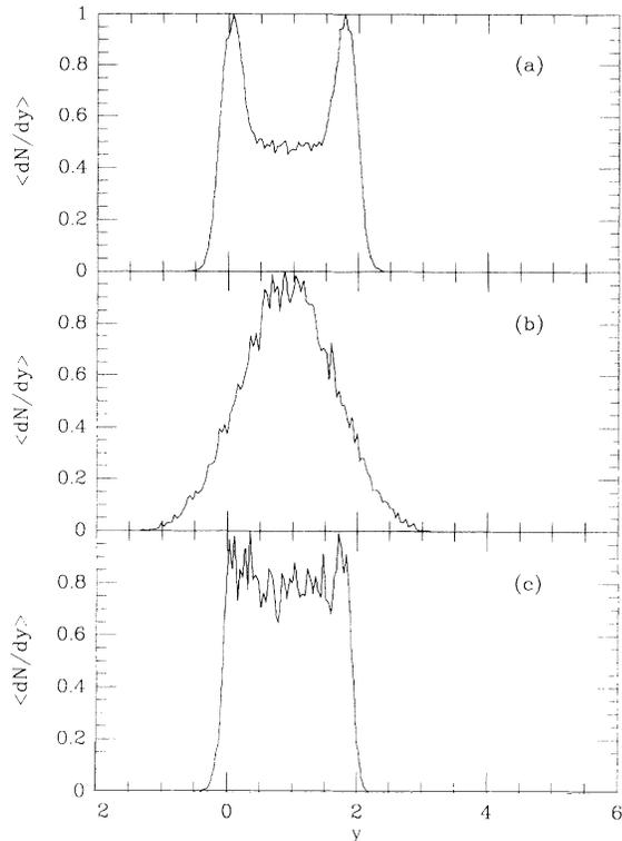
FIG. 11. Distributions of the rapidity  $y = \frac{1}{2} \ln \frac{E+p_{\parallel}}{E-p_{\parallel}}$ . For the reaction Ar+Ar at 2 GeV per nucleon we analyzed (a) the nucleons (free and bound), (b) the pions, and (c) the fragments in the final state. Normalization is arbitrary.
