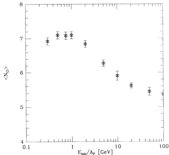
FIG. 5. Average number of stable fragments in the final state of the reaction Ar+Ar (regardless of the number of nucleons contained in one cluster). Error bars mark the uncertainty in the average and not the deviation of single values.
