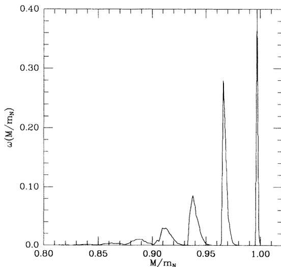
FIG. 2. Distribution for the effective masses ( $M = \sqrt{p_i^2}$ ) in the reaction Ar+Ar at 2 GeV per nucleon at that instant where we find the greatest number of interactions. The originally discret values are contracted and smeared out due to the factor introduced in (3.17). We normalized  $\omega(M/m_N)$  to the value at  $M/m_N = 1$  (not included in the figure).
