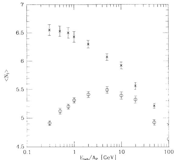
FIG. 6. Maximum number of simultaneous interactions that any nucleon had at any stage of the reaction Ar+Ar. This measure for the local nuclear density obviously increases by increasing the depth of the quasipotential (circles:  $V_0 = 0$  MeV, crosses:  $V_0 = 60$  MeV). Error bars mark the uncertainty in the average and not the deviation of single values.
