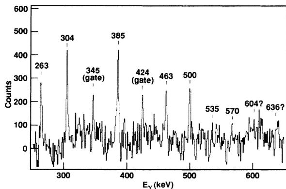
FIG. 1. Spectrum obtained with single gates on the clean SD band transitions at 345 and 424 keV in  $^{192}\text{Pb}$ . These data are from our original thin target experiment which used the  $^{173}\text{Yb}(^{24}\text{Mg},5n)$  reaction at 132 MeV. Clearly evident are all the SD band members through the 500-keV transition reported in Ref. [1].
