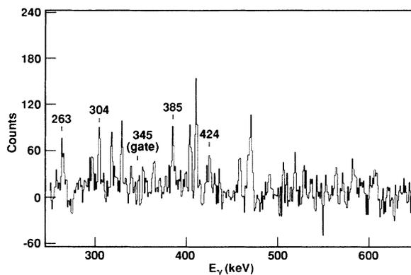
FIG. 2. Spectrum obtained with a single gate on the SD band transition at 345 keV. These data are from the  $^{148}\text{Sm}(^{48}\text{Ca}, 4n)$  reaction at 205 MeV with a gold backed target. Although no longer completely clean, the SD band is still clearly observed; transitions above about 450 keV are expected to be significantly Doppler broadened or shifted.
