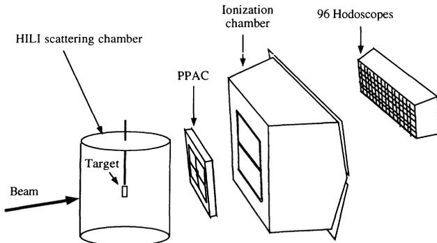
FIG. 1. Schematic view of the HILI (heavy-ion-light-ion) detection system.
