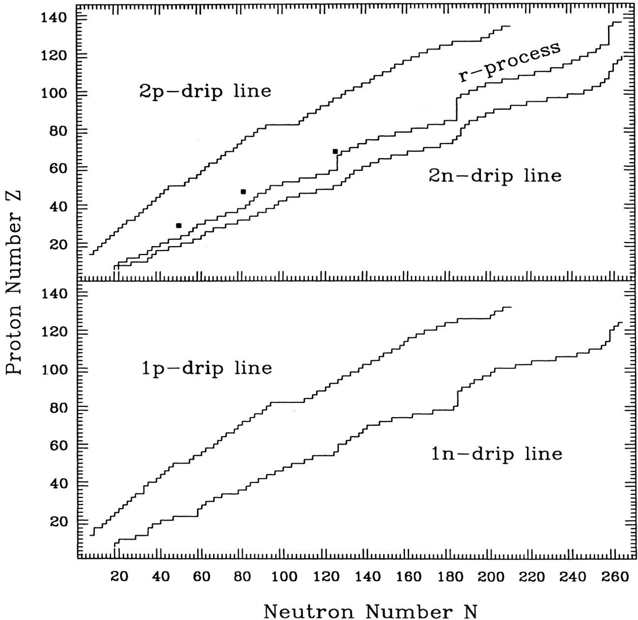
FIG. 1. One-particle (bottom) and two-particle (top) neutron and proton drip lines obtained within the HFB theory with the SkP Skyrme interaction. The middle line in the top part of the figure corresponds to an approximated  $r$ -process path. Three full squares represent positions of the three nuclides being at the origin of abundance maxima, i.e.,  $^{80}_{30}\text{Zn}_{50}$ ,  $^{130}_{48}\text{Cd}_{82}$ , and  $^{195}_{69}\text{Tm}_{126}$ .
