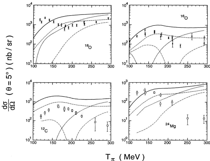
FIG. 3. Data are the same as Fig. 2. Solid and dashed curves result from calculations combining DINT and SEQ contributions from Fig. 2. Dotted and dot-dashed use the same amplitude, but with the DINT-SEQ phase arbitrarily set to  $180^\circ$ .
