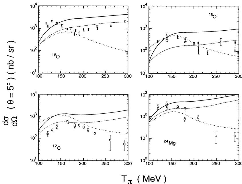
FIG. 2. Pion double charge-exchange g.s.  $\rightarrow$  g.s. cross sections (at  $5^\circ$ ) vs  $T_\pi$  for one  $T = 1$  and three  $T = 0$  nuclei. Solid and dashed curves are  $j_{\text{pair}} = 0$  SEQ calculations, full and orbit nonchanging, respectively. Dotted curves are DINT calculations.
