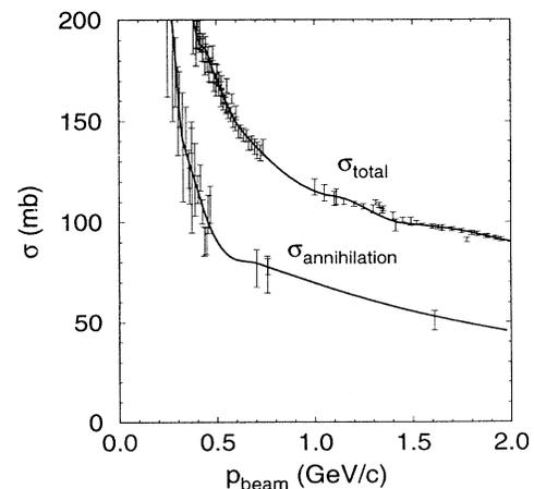
FIG. 1. Antiproton-proton total and annihilation cross-sections as a function of beam momentum [14].
