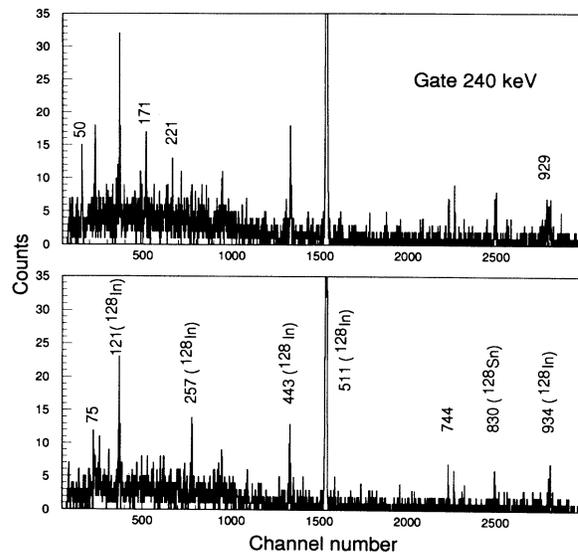
FIG. 12. Gate on the 240 keV peak, in the  $\gamma$ - $\gamma$  coincidences, from the  $^{32}\text{Na}$  decay, establishes the cascade relations of the set of levels revealed by the  $n, \gamma$  coincidences (background in the lower part of the figure).
