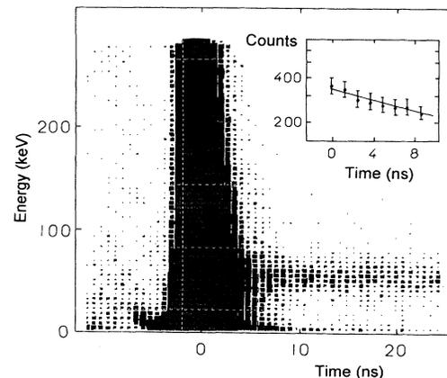
FIG. 2. Delayed coincidences taken in the decay of  $^{31}\text{Na}$  with the NE102 plastic  $\beta$  detector and a small  $\text{BaF}_2$  scintillator. In the inset the decay curve of the 50 keV gate, a least-squares fit leads to the value of  $T_{1/2} = 16.0 \pm 2.8$  ns.
