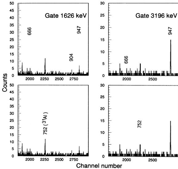
FIG. 8. Upper left: gate on the 1626 keV line emphasizing the components of the  $4143 \rightarrow 3239 \rightarrow 947 \rightarrow 0$  cascade (background below). Upper right: gate on the 3196 keV line showing the outstanding presence of the 947 keV transition, whereas the 666 keV peak does not exhibit the expected strength if the 3196 keV ray assignment of Ref. [20] is assumed. However, a weak contribution of this process cannot be excluded.
