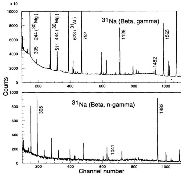
FIG. 5. Partial  $\gamma$  spectrum of the  $^{31}\text{Na}$  ( $\beta, \gamma$ ) decay is shown in the top part of the figure and compared in the same energy range to the spectrum taken in coincidence with neutrons in the bottom part. Note the enhancement of the  $\gamma$  lines subsequent to the  $1n$  process; lines arising in the  $2n$  process (e.g., 1041 keV) are not substantially favored by the coincidence technique, probably because of the energy threshold in the neutron detection chain.
