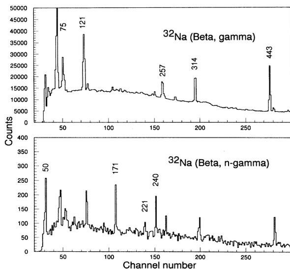
FIG. 11. Comparison of the direct  $\gamma$  spectrum of the  $^{32}\text{Na}$  ( $\beta, \gamma$ ) process to the  $\gamma$  spectrum taken in coincidence with neutrons. The enhancement of the lines at 171, 221, 240, and 929 keV (not shown) provides a clear evidence for the population of a set of levels in  $^{31}\text{Mg}$  distinct from those populated in the  $^{31}\text{Na}$  decay.
