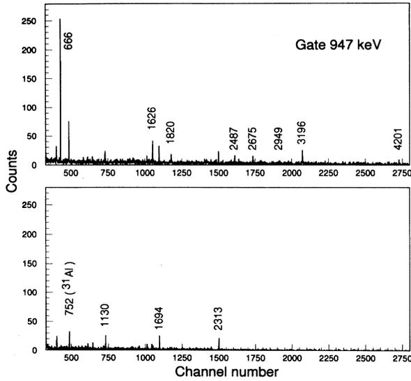
FIG. 7. Gate on the 947 keV line corresponding to the deexcitation of the first level in  $^{31}\text{Al}$ . The lower part of the figure shows the corresponding background. These results support the whole framework of the proposed  $^{31}\text{Mg}$  decay scheme.
