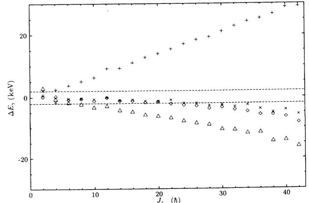
FIG. 3. Differences in  $\gamma$ -ray energies  $\Delta E_\gamma$  between the  $A = 194$  bands and the <sup>192</sup>Hg band. The bands are represented by + (<sup>194</sup>Pb), × (<sup>194</sup>Pb\*), △ (<sup>194</sup>Hg), and ◇ (<sup>194</sup>Hg\*). The two dashed lines at  $\pm 2$  keV represent the accuracy required experimentally for twinning.
