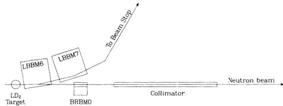
FIG. 1. Layout of BR neutron-production beam line at LAMPF. The primary proton beam is swept aside by LBBM6 and 7. The neutron beam is precessed by the fringes of LBBM6 and 7 and by BRBM0.
