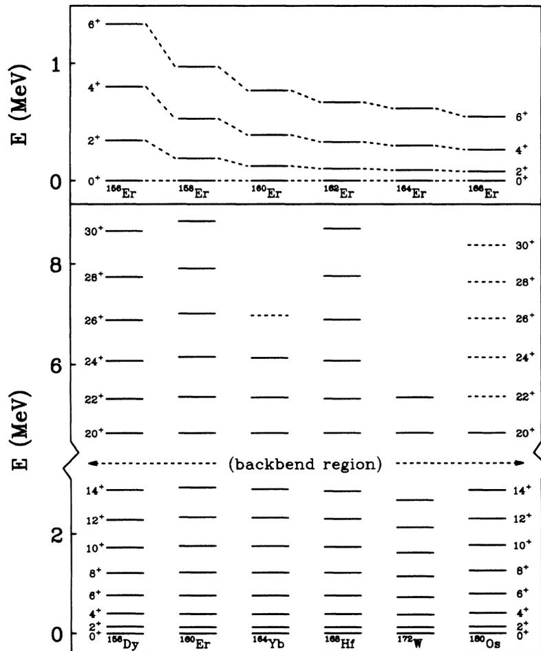
FIG. 1. Top: Low spin yrast levels [11] of  $^{156-166}\text{Er}$  showing a shape transitional region. Bottom: Levels of the multiplet  $^{156}\text{Dy}-^{180}\text{Os}$  showing the occurrence of nearly identical band spacings. The backbending region, of course, differs in detail in these nuclei and is excluded from the comparison. Above the backbend, the energies are normalized to  $^{156}\text{Dy}$  at spin  $20^+$  to emphasize the rotational spacings.
