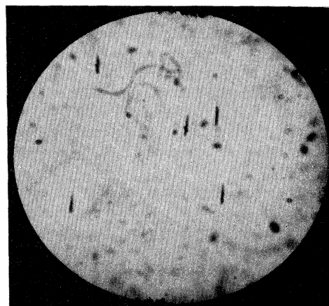
FIG. 2. Photomicrograph of the oriented fission fragment tracks in lexan from the 65 MeV He-ion-induced fission of ^{165}\text{Ho} .
