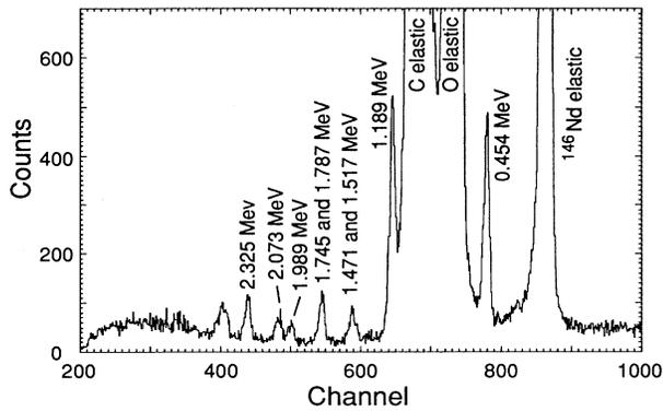
FIG. 1. Spectrum of scattered protons taken at a laboratory angle of  $35^\circ$ . Peaks corresponding to states in  $^{146}\text{Nd}$  are labeled with their excitation energies. The large peaks corresponding to elastic scattering from carbon and oxygen nuclei are clearly evident.
