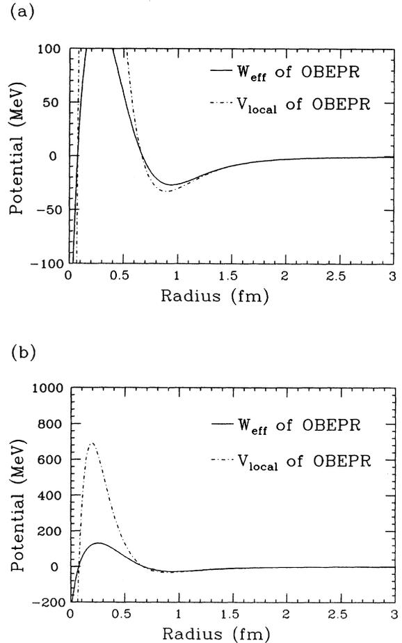
FIG. 3. A comparison between the full OBEPR effective local  $^3S_1$  potential at the deuteron energy and that obtained by removing the  $p^2$  terms, without any other changes to the model. Differences are small on the scale of (a). The effect of removing the  $p^2$  terms on the deuteron is to weaken its binding energy to a value of 0.8 MeV. The effect of the  $p^2$  terms is seen to be more appreciable in (b), where the same curves are graphed on a larger scale.
